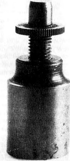
An easily-made screw-jack which can prove extremely useful when adjusting work being clamped down.
