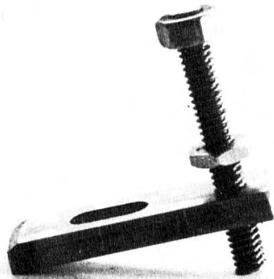
A typical clamping bar with adjusting bolt. The inclusion of this bolt saves the constant search for packing when clamping work.
