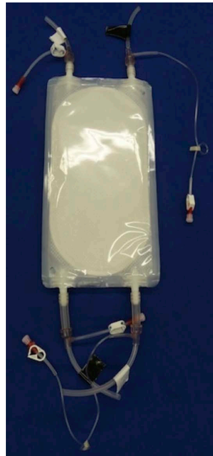
FIGURE 2. FO Urine-to-Water Processing Bag Tested on STS-135
