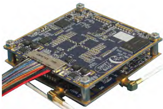
Figure 17. SWIFT-RelNav Radio Prototype. TUI’s SWIFT-RelNav radio provides cross-link communications at up to 12 Mbps in addition to range and direction tracking.
