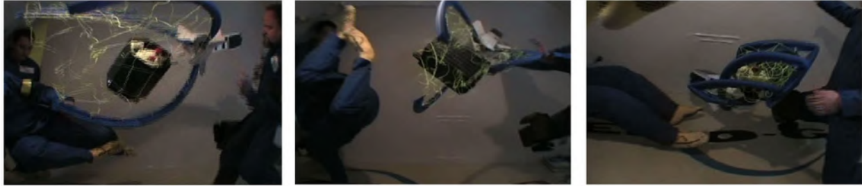
Figure 20. Microgravity Test of GRASP Prototype. GRASP provides a scalable solution capable of capturing tumbling objects.
