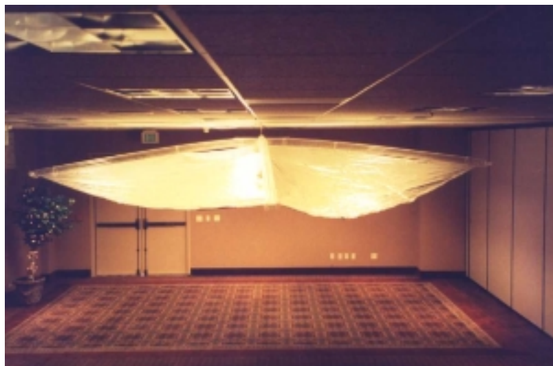
Figure 16. A Pioneer Astronautics Inflatable Boom Solar Sail Deployed in a Hotel Ballroom
