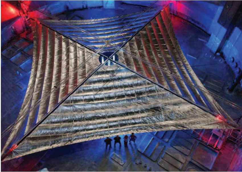
Figure 12.3. The L’Garde solar sail before vacuum testing at NASA’s Plum Brook facility. The scale of the device can be appreciated by examining the relative size of the people in front of it. (Courtesy of NASA) (See also color insert.)
