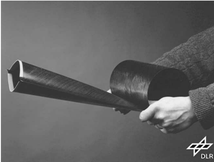
Figure 11.2. This rigid boom was used by DLR to deploy its solar sail during ground testing in 1999. (Courtesy of DLR)
