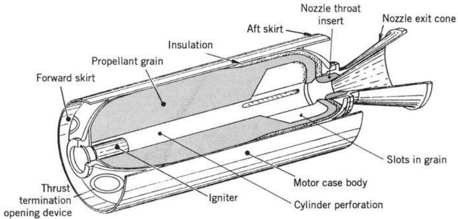
**FIGURE 1-5.** Simplified perspective three-quarter section of a typical solid propellant rocket motor with the propellant grain bonded to the case and the insulation layer and with a conical exhaust nozzle. The cylindrical case with its forward and aft hemispherical domes form a pressure vessel to contain the combustion chamber pressure. Adapted with permission from Reference 11-1.
