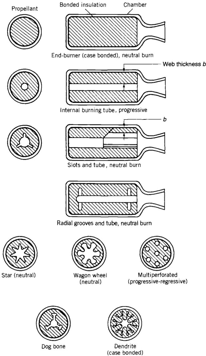
FIGURE 11-16. Simplified diagrams of several grain configurations.
