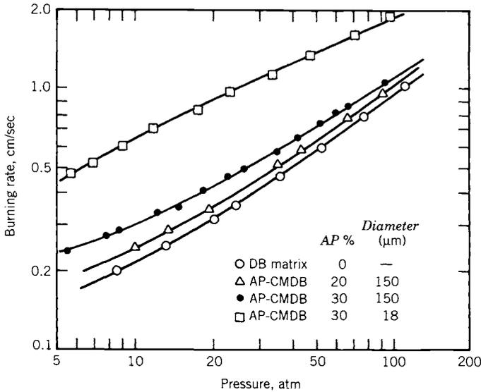
**FIGURE 11-7.** Measured burning rate characteristics of a double-base (DB) propellant and three composite-modified double-base (CMDB) propellants which contain an increasing percentage of small diameter (159 μm) particles of ammonium perchlorate (AP). When the size of the AP particles is reduced or the percentage of AP is increased, an increase in burning rate is observed. None of these data form straight lines. (Reproduced with permission of the AIAA from Chapter 1 of Ref. 11-3.)
