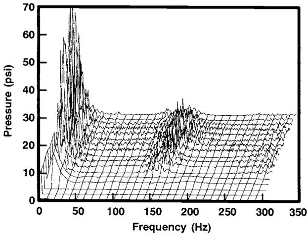
**FIGURE 15-12.** A frequency-versus-amplitude plot at successive time intervals for an 11-in. diameter GOX/HTPB motor test shows pressure oscillations in the motor 1-L acoustic mode at 150 Hz due to flame-holding instability.
