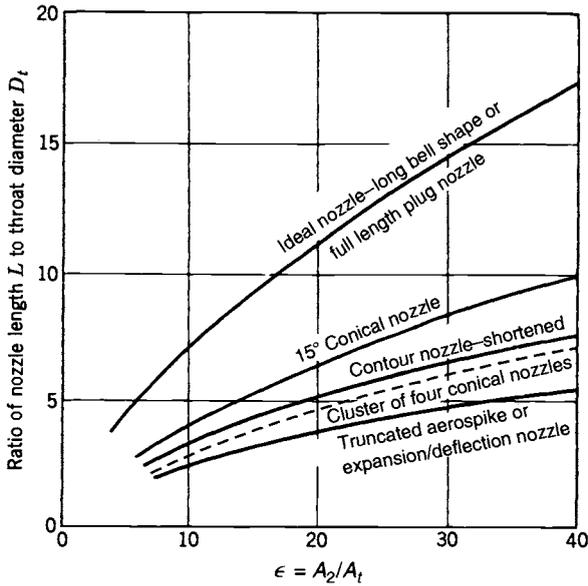
**FIGURE 3-13.** Length comparison of several types of nozzles. (Taken in part from G. V. R. Rao, "Recent Developments in Rocket Nozzle Configurations," American Rocket Society Journal, Vol. 31, No. 11, November 1961.)
