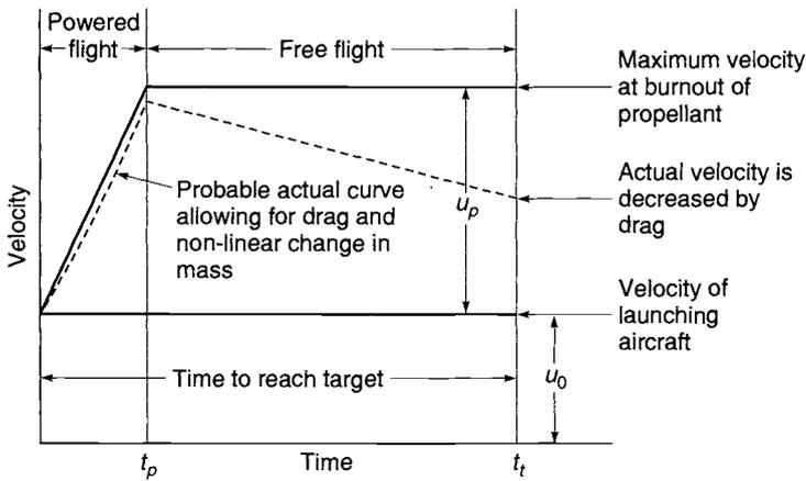
**FIGURE 4-17.** Simplified trajectory for an unguided, non-maneuvering, air-launched rocket projectile. Solid line shows flight velocity without drag or gravity and dashed curve shows likely actual flight.
