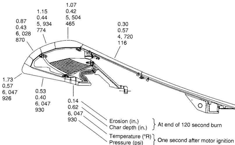
**FIGURE 14-10.** Erosion measurements and char depth data of the carbon fiber phenolic material of the nozzle of the Space Shuttle reusable solid rocket motor. (Courtesy of Thiokol Propulsion, a Division of Cordant Technologies.)
