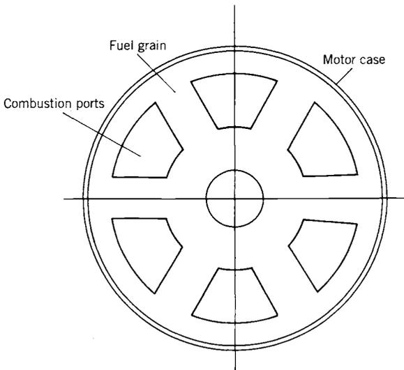
**FIGURE 15-5.** Cross-sectional sketch of a multi-port fuel grain with web thickness between ports twice that of the outer wall. Multiple ports are required to achieve the large fuel surface area necessary for high fuel flow rates.
