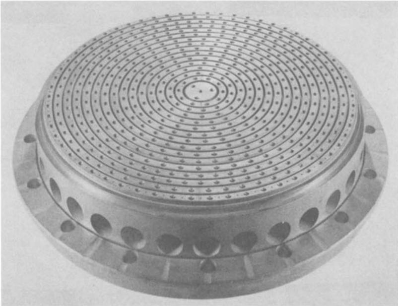
**FIGURE 8-4.** Injector with  $90^\circ$  self-impinging (fuel-against-fuel and oxidizer-against-oxidizer)-type countersunk doublet injection pattern. Large holes are inlets to fuel manifolds. Pre-drilled rings are brazed alternately over an annular fuel manifold or groove and a similar adjacent oxidizer manifold or groove. A section through a similar but larger injector is shown in Fig. 8-1.
