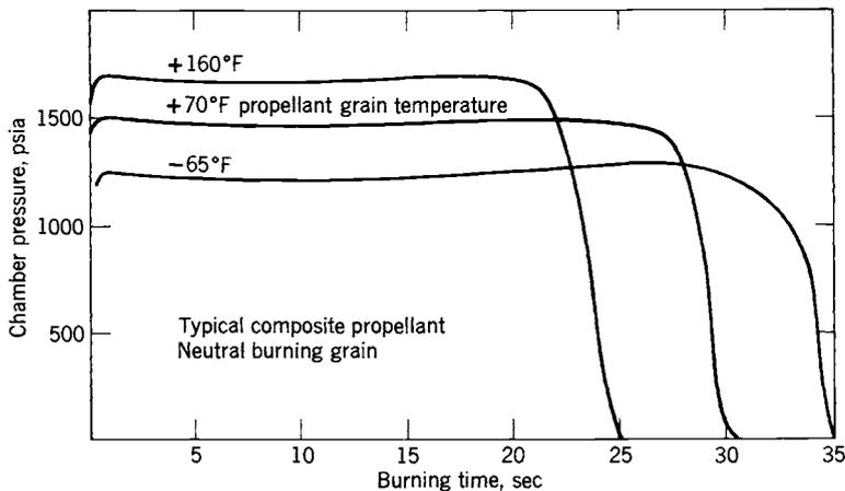
**FIGURE 11-8.** Effect of propellant temperature on burning time and chamber pressure for a particular motor. The integrated areas under the curves are proportional to the total impulse, which is the same for the three curves.
