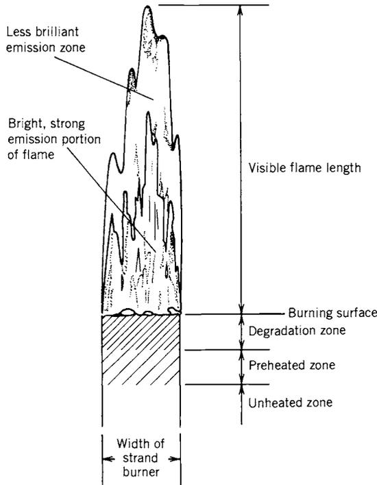
**FIGURE 13-2.** Diagram of the flickering, irregular combustion flame of a composite propellant (69% AP, 19% Al, plus binder and additives) in a strand burner with a neutral atmosphere. (Adapted from Chapter 1 of Ref. 13-1 with permission of AIAA.)
