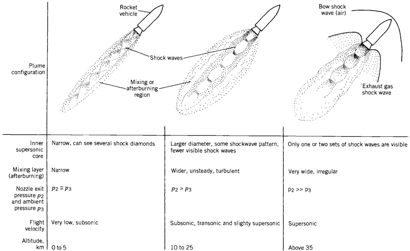
**FIGURE 18-2.** The visible plume grows in length and diameter as the rocket vehicle gains altitude. The afterburning of the fuel-rich combustion products with the oxygen from the air occurs in the mixing layer. At very high altitude, above perhaps 200 km, there is no air and therefore no afterburning.
