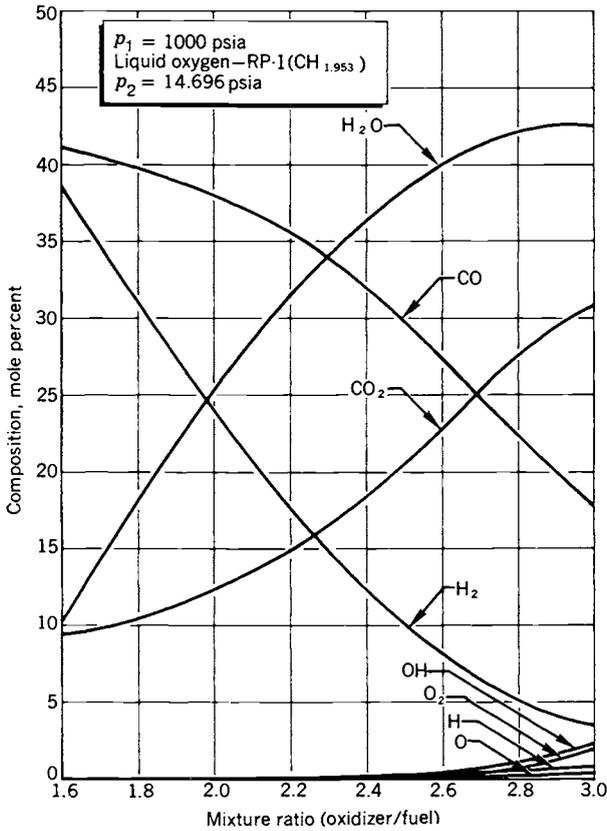
FIGURE 5-3. Calculated nozzle exit gas composition for shifting equilibrium conditions as a function of mixture ratio. Breakdown into O, OH, or H and free  $\text{O}_2$  occurs only at the higher temperatures or higher mixture ratios.
