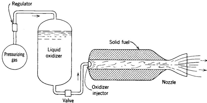
**FIGURE 1-6.** Simplified schematic diagram of a typical hybrid rocket engine. The relative positions of the oxidizer tank, high pressure gas tank, and the fuel chamber with its nozzle depend on the particular vehicle design.
