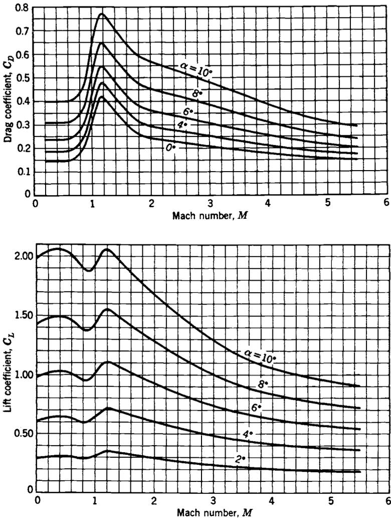
**FIGURE 4-3.** Variation of lift and drag coefficient with Mach number of the German V-2 missile based on body cross-sectional area with jet off and without exhaust plume effects at several angles of attack  $\alpha$ .
