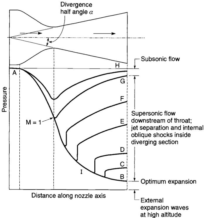
**FIGURE 3-9.** Distribution of pressures in a converging-diverging nozzle for different flow conditions. Inlet pressure is the same, but exit pressure changes. Based on experimental data from A. Stodala.
