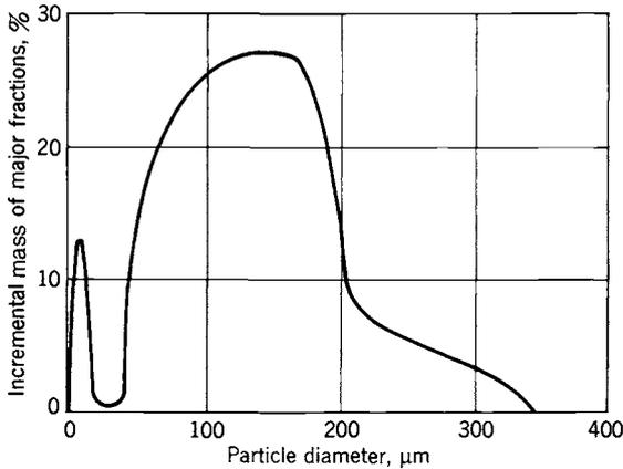
**FIGURE 12-10.** The oxidizer (AP) particle size distribution is a blend of two or more different particle sizes; this particular composite propellant consists of a narrow cut at about 10  $\mu\text{m}$  and a broad region from 50 to 200  $\mu\text{m}$ .
