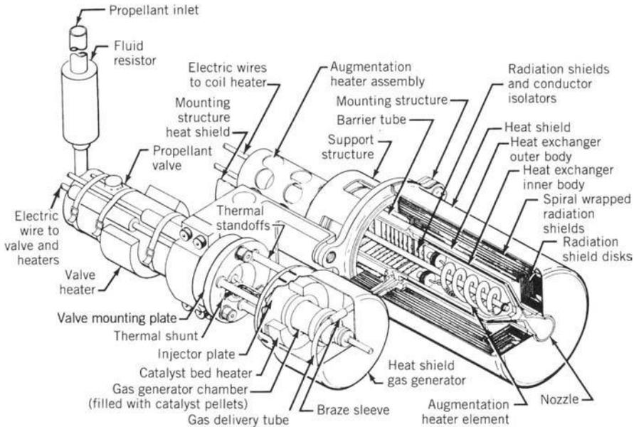
**FIGURE 19-4.** Resistojet augmented by hot gas from catalytically decomposed hydrazine; two main assemblies are present: (1) a small catalyst bed with its electromagnetically operated propellant valve and heaters to prevent hydrazine from freezing, and (2) an electrical resistance spiral-shaped heater surrounded by thin radiation shields, a refractory metal exhaust nozzle, and high-temperature electrical insulation supporting the power leads. (Courtesy of PRIMEX Aerospace Company.)
