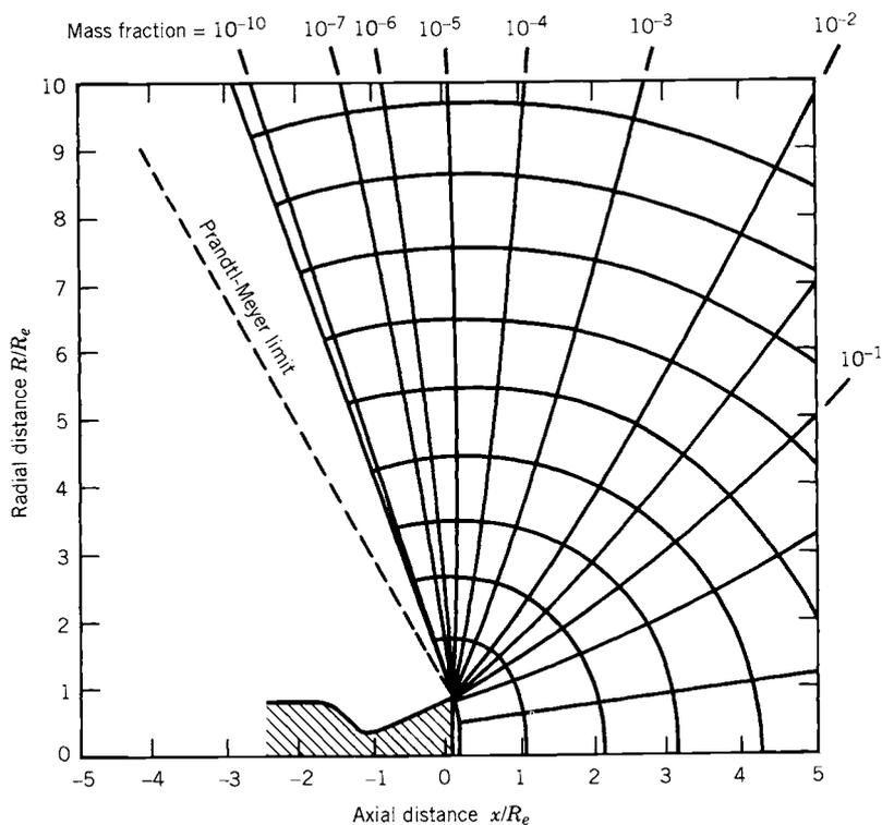
**FIGURE 18-3.** Density profile for vacuum plume expansion using a one-dimensional flow model for a small storable bipropellant thruster. The axial distance  $x$  and the plume radius  $R$  have been normalized with the nozzle exit radius  $R_e$ . Here  $k = 1.25$ , the Mach number of the nozzle exit is 4.0, and the nozzle cone half angle is  $19^\circ$ .
