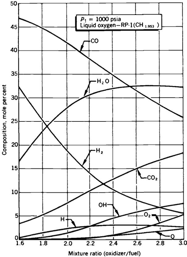
**FIGURE 5-2.** Calculated chamber gas composition for liquid oxygen and hydrocarbon fuel as a function of mixture ratio. Aggressive gases, such as  $\text{O}_2$ ,  $\text{O}$ , or  $\text{OH}$ , can cause oxidation of the wall materials in the chamber and the nozzle.
