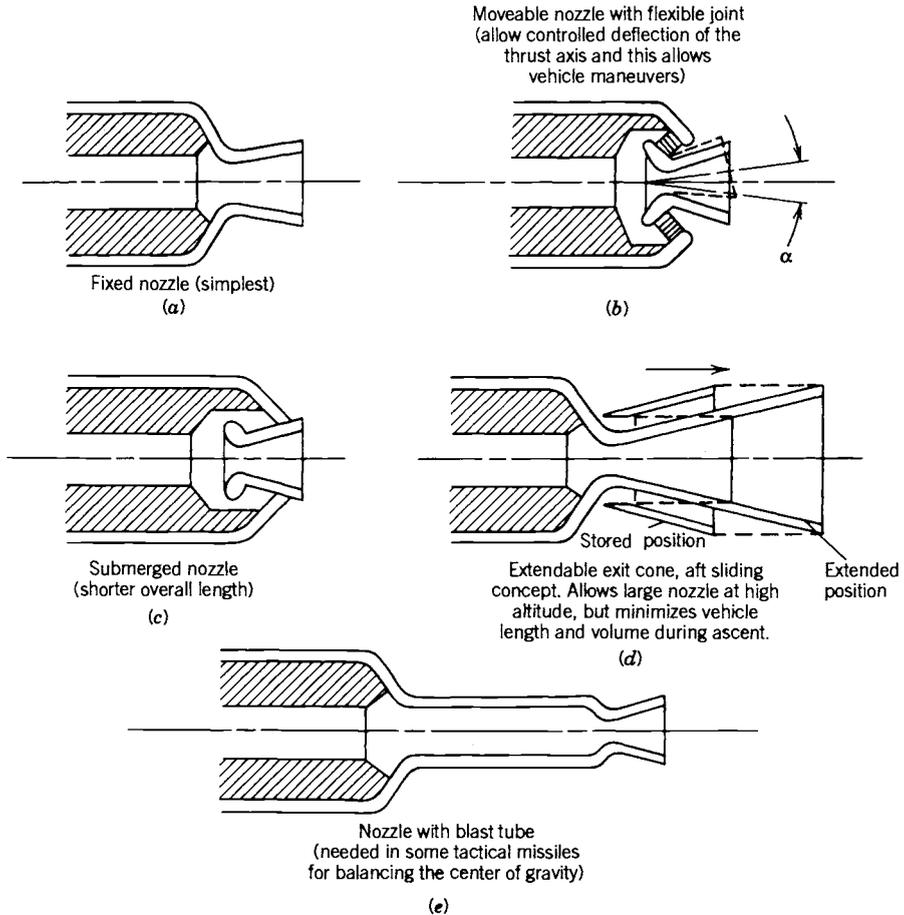
FIGURE 14-6. Simplified diagrams of five common nozzle configurations.
