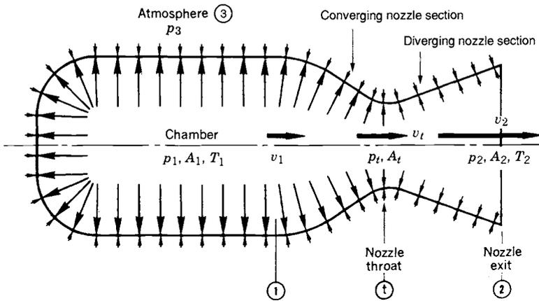
**FIGURE 2-1.** Pressure balance on chamber and nozzle interior walls is not uniform. The internal gas pressure (indicated by length of arrows) is highest in the chamber ( $p_1$ ) and decreases steadily in the nozzle until it reaches the nozzle exit pressure  $p_2$ . The external or atmospheric pressure  $p_3$  is uniform. At the throat the pressure is  $p_t$ . The four subscripts (shown inside circles) refer to the quantities  $A$ ,  $v$ ,  $T$ , and  $p$  at specific locations.
