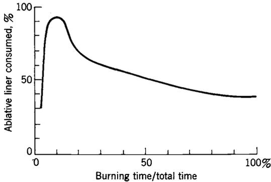
**FIGURE 8-10.** Relative depth of pyrolysis of ablative material with different duty cycles using many short-duration thrust pulses for a small liquid propellant reaction control thrust chamber of 20 lbf thrust.
