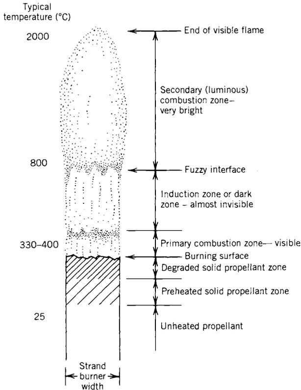
**FIGURE 13-1.** Schematic diagram of the combustion flame structure of a double-base propellant as seen with a strand burner in an inert atmosphere. (Adapted from Chapter 1 of Ref. 13-1 with permission of the American Institute of Aeronautics and Astronautics, AIAA.)
