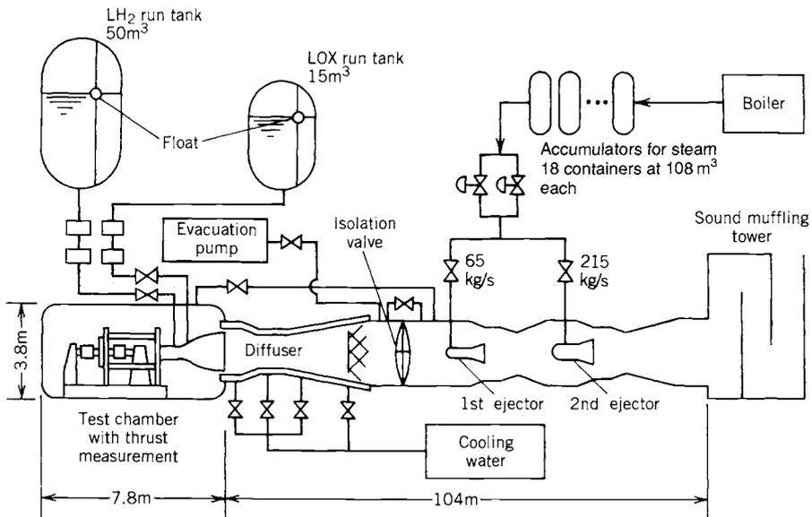
**FIGURE 20-2.** Simplified diagram of a simulated altitude, horizontal firing test facility for the LE-5 Japanese-designed thrust chamber (liquid oxygen–liquid hydrogen propellants) showing the method of creating a vacuum (6 torr during operation and 13 torr prior to start). The operating duration is limited to about 10 min by the capacity of the steam storage. (Reproduced from Ref. 20-1 with permission of the AIAA.)
