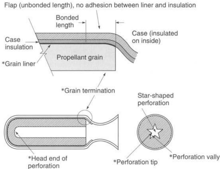
**FIGURE 11–24.** The asterisks in the bottom simplified diagram denote potentially critical failure areas. The top sketch is an enlargement of the aft termination region of the grain and shows a boot or stress relief flap.
