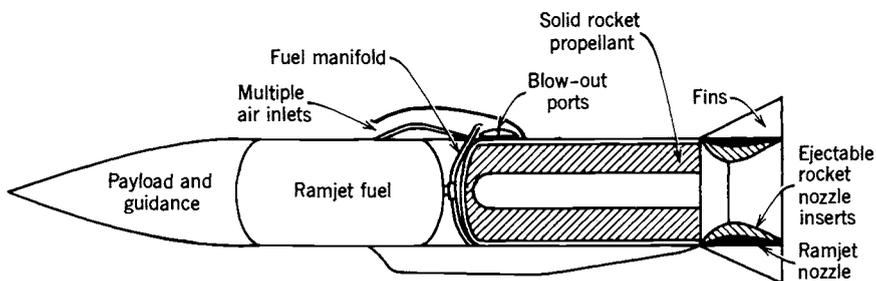
**FIGURE 1-7.** Elements of an air-launched missile with integral rocket-ramjet propulsion. After the solid propellant has been consumed in boosting the vehicle to flight speed, the rocket combustion chamber becomes the ramjet combustion chamber with air burning the ramjet liquid fuel.
