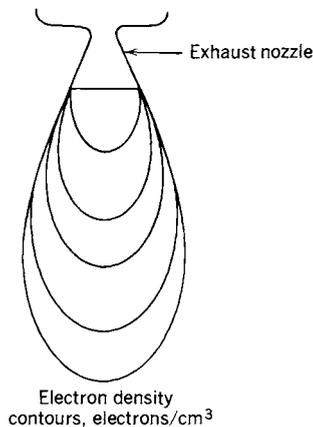
**FIGURE 18–8.** Exhaust plume model for predicting attenuation of radio communications signals. The contours shown are for either equal electron density or electron collision frequency; the highest values are near the nozzle exit.
