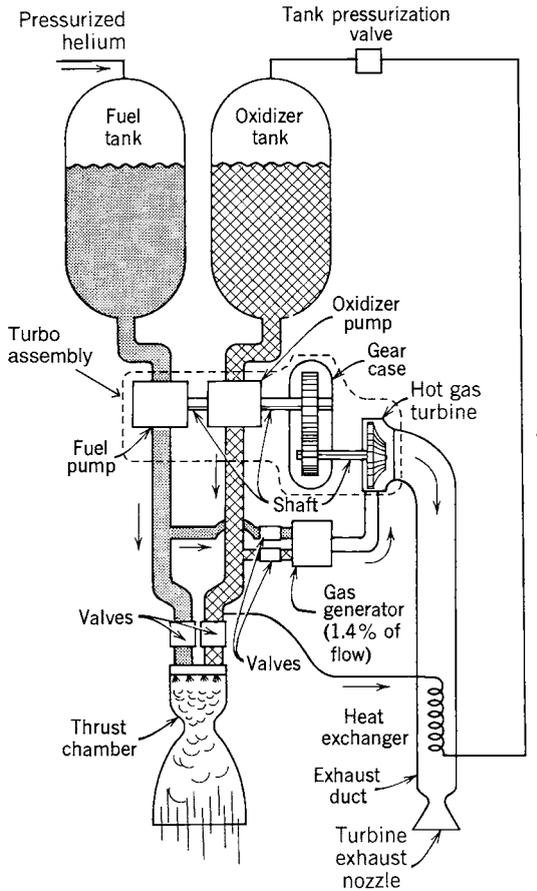
**FIGURE 1-4.** Simplified schematic diagram of one type of liquid propellant rocket engine with a turbopump feed system and a separate gas generator, which generates warm gas for driving the turbine. Not shown are components necessary for controlling the operation, filling, venting, draining, or flushing out propellants, filters or sensors. The turbopump assembly consists of two propellant pumps, a gear case, and a high speed turbine.
