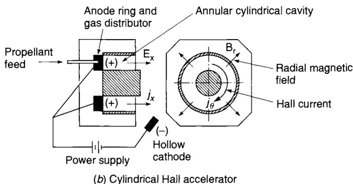
**FIGURE 19–10.** Linear and cylindrical Hall accelerator configurations showing how an applied axial field results in a transverse current that accelerates the plasma. The Hall current peaks when the external resistance is absent (i.e., shorted). The presence of any significant axial current density  $j_x$  represents an inefficiency in Hall devices.
