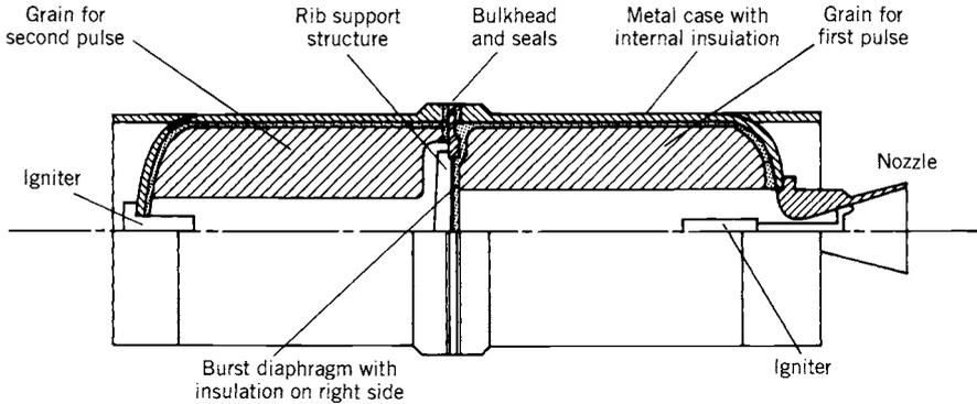
**FIGURE 11-20.** Simplified diagram of one concept of a two-pulse experimental rocket motor with two grains separated by a bulkhead. During the first pulse operation the metal diaphragm is supported by a spider-web-like structure made of high temperature material. Upon ignition of the second stage, the scored diaphragm is loaded in the other direction; it breaks and its leaves peel back. The bulkhead opening has a much larger area than the nozzle throat.
