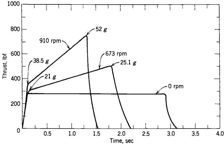
**FIGURE 11-12.** Effect of axial spin on the thrust-time behavior of a rocket motor with composite propellant using aluminum and PBAN (polybutadiene acrylonitrile) as fuels. (Adapted with permission from Ref. 11-7.)
