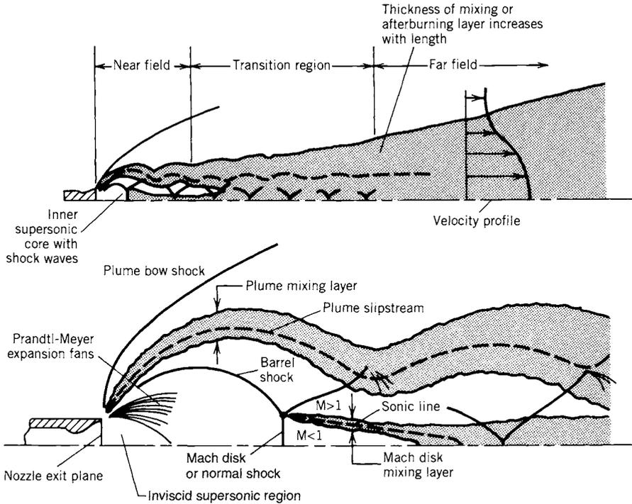
**FIGURE 18-1.** Half sections of schematic diagrams of a rocket exhaust plume at low altitude. Upper sketch shows full plume and lower sketch is an enlargement of the near field. (Reprinted with permission from Ref. 18-1.)
