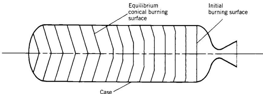
**FIGURE 11-18.** Schematic diagram of end-burning grain coning effect. In larger sizes (above approximately 0.5 m diameter) the burning surface does not remain flat and perpendicular to the motor axis, but gradually assumes a conical shape. The lines in the grain indicate successively larger-area burning surface contours.
