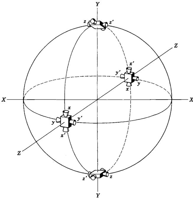
**FIGURE 4-13.** Simplified attitude control system diagram for spacecraft. It requires 12 thrusters (identified as  $x$ ,  $y$ ,  $z$ ) to allow the application of pure torques about three perpendicular axes. The four unlabeled thrusters are needed for translation maneuvers along the  $z$  axis. They are shown here in four clusters.
