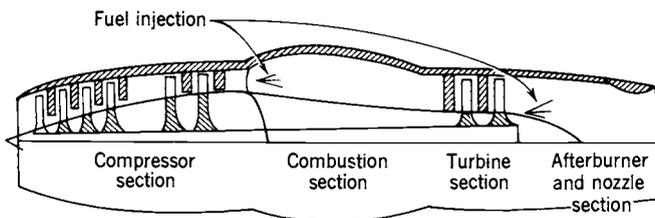
FIGURE 1-1. Simplified schematic diagram of a turbojet engine.
