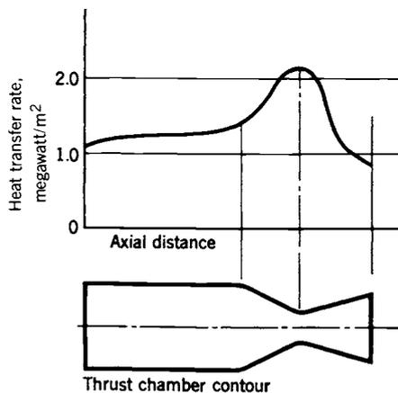
**FIGURE 8-8.** Typical axial heat transfer rate distribution for liquid propellant thrust chambers and solid propellant rocket motors. The peak is always at the nozzle throat and the lowest value is usually near the nozzle exit.
