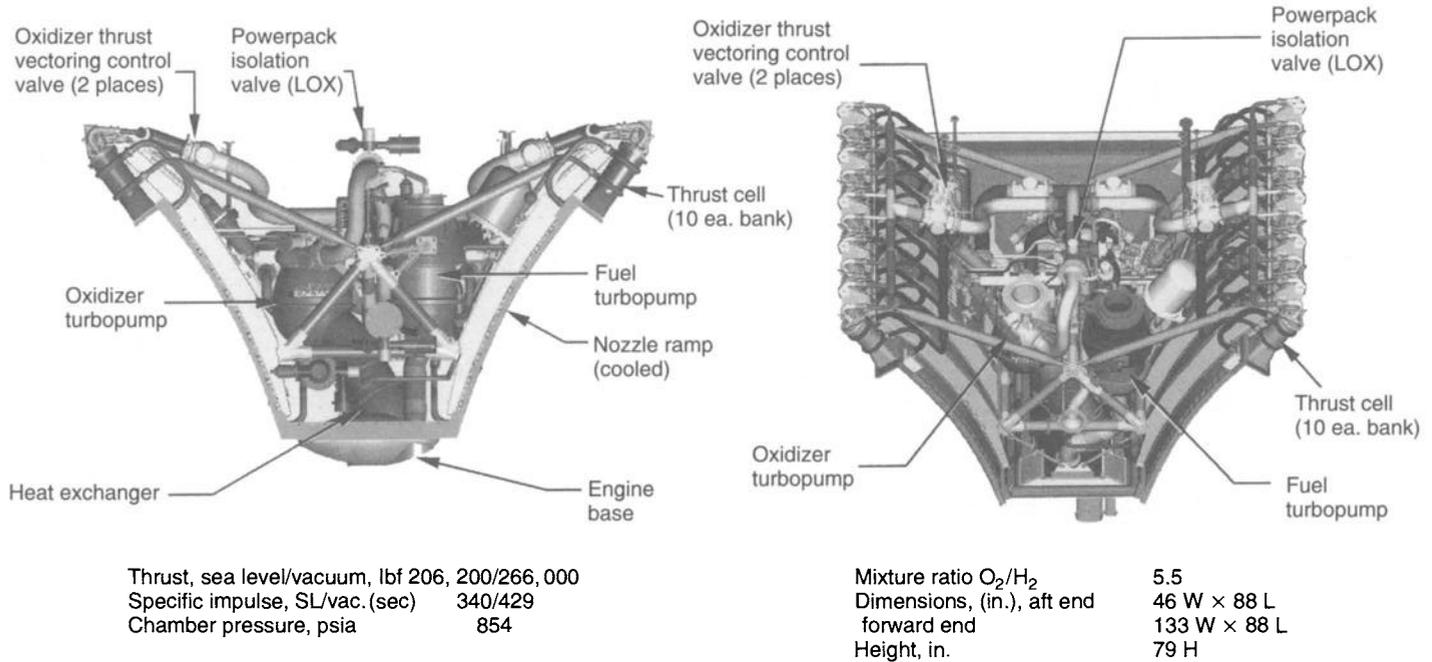
**FIGURE 8-13.** Side view and oblique top view of the XRS-2200 aerospike linear rocket engine with 20 thrust cells and two curved fuel-cooled ramps. (Courtesy of The Boeing Company, Rocketdyne Propulsion and Power.)
