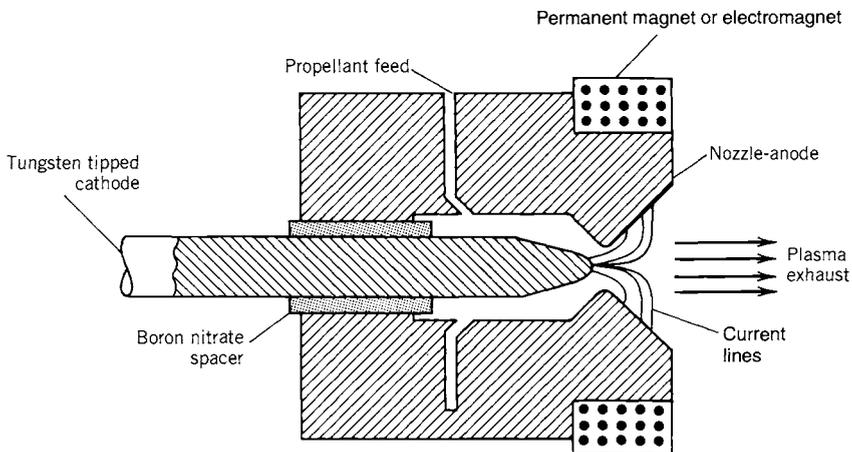
**FIGURE 19-9.** Simplified diagram of a magnetoplasmadynamic (MPD) arcjet thruster. It is similar in construction to the thermal arcjet shown in Fig. 1-8 but it has a stronger magnetic field to enhance the propellant acceleration.
