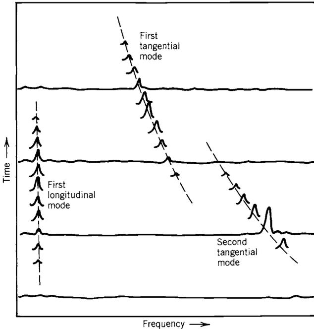
**FIGURE 13-6.** Example of mode frequency display; also called a “waterfall” diagram of a motor firing. Only four complete time–frequency curves are shown; for easy visualization the other time lines are partly omitted except near the resonating frequencies. The height of the wave is proportional to pressure. As the cavity volume increases, the frequencies of the transverse modes decrease. (Adapted from E. W. Price, Chapter 13 of Ref. 13-1, with permission of AIAA.)
