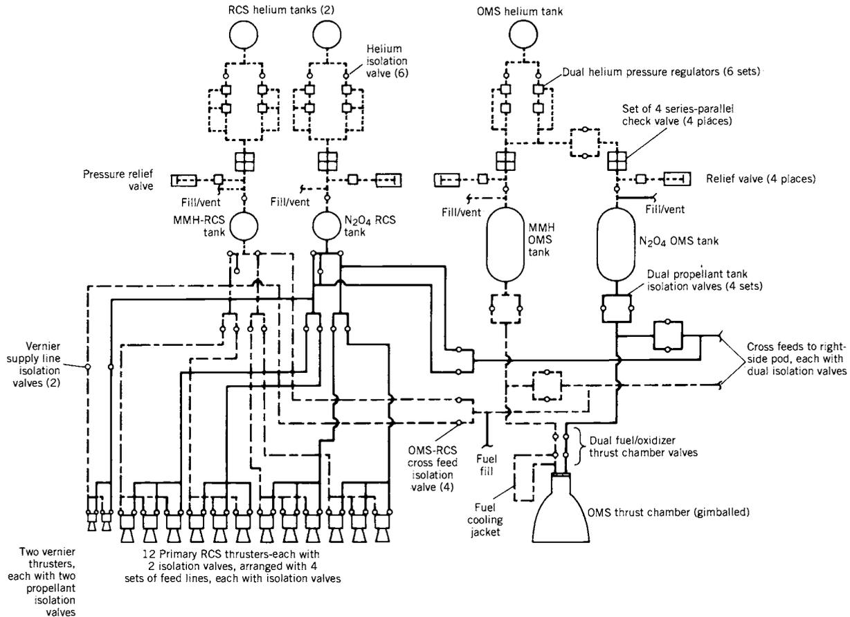
**FIGURE 6-4.** Simplified flow diagram of the propellant feed system flow for the left aft pod of the Orbital Maneuvering System (OMS) and Reaction Control System (RCS) of the Space Shuttle Orbiter Vehicle. Solid lines: nitrogen tetroxide (N<sub>2</sub>O<sub>4</sub>); dash-dot lines: monomethylhydrazine (MMH); short dashed lines: high-pressure helium. (Source: NASA.)
