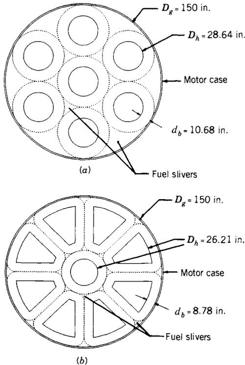
**FIGURE 15-9.** (a) Circular fuel grain combustion ports are volumetrically inefficient and leave large slivers at burnout. (b) Quadrilateral port hybrid grain configuration minimizes residual fuel sliver at burnout.
