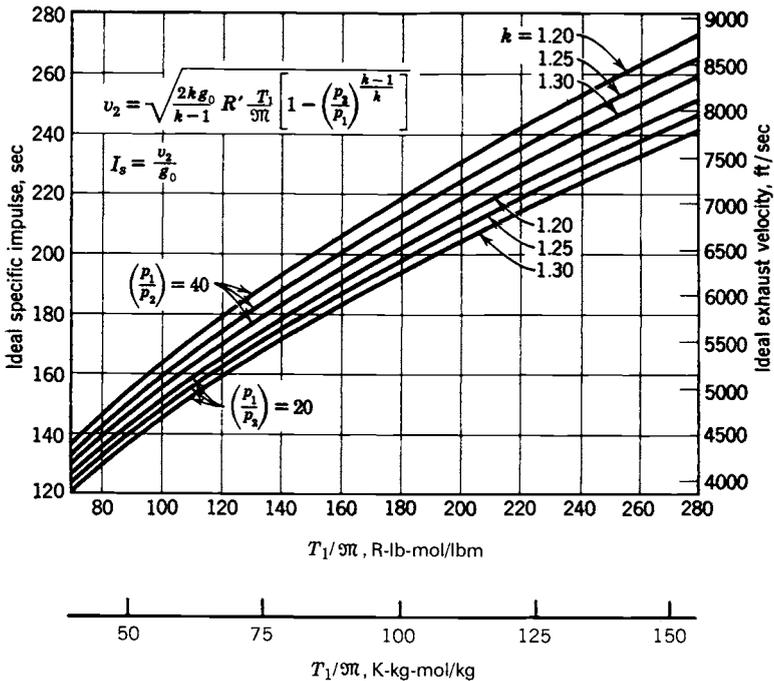
**FIGURE 3-2.** Specific impulse and exhaust velocity of an ideal rocket at optimum nozzle expansion as functions of the absolute chamber temperature  $T_1$  and the molecular mass  $\mathfrak{M}$  for several values of  $k$  and  $p_1/p_2$ .
