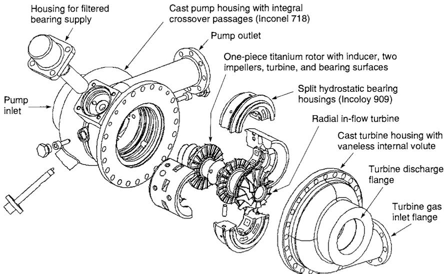
**FIGURE 10-2.** Exploded view of an advanced high-speed, two-stage liquid hydrogen fuel pump driven by a radial flow turbine. (Copied with permission of Pratt & Whitney, a division of United Technologies; adapted from Ref. 10-2.)
