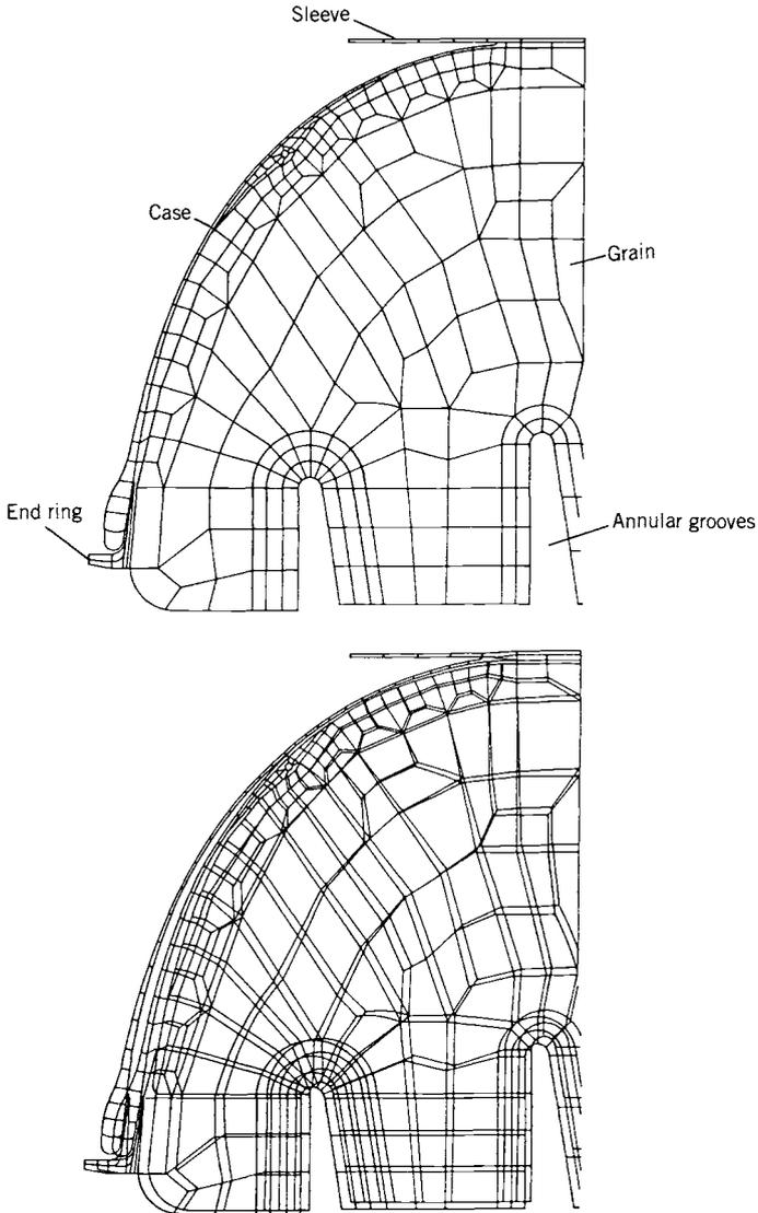
**FIGURE 11-22.** Finite element analysis grid of the forward end of a cast grain in a filament-wound plastic case. The grain has an internal tube and annular grooves. The top diagram shows the model grid elements and the bottom shows one calculated strain or deformation condition. (Reprinted with permission from A. Turchot, Chapter 10 of Ref. 11-1).
