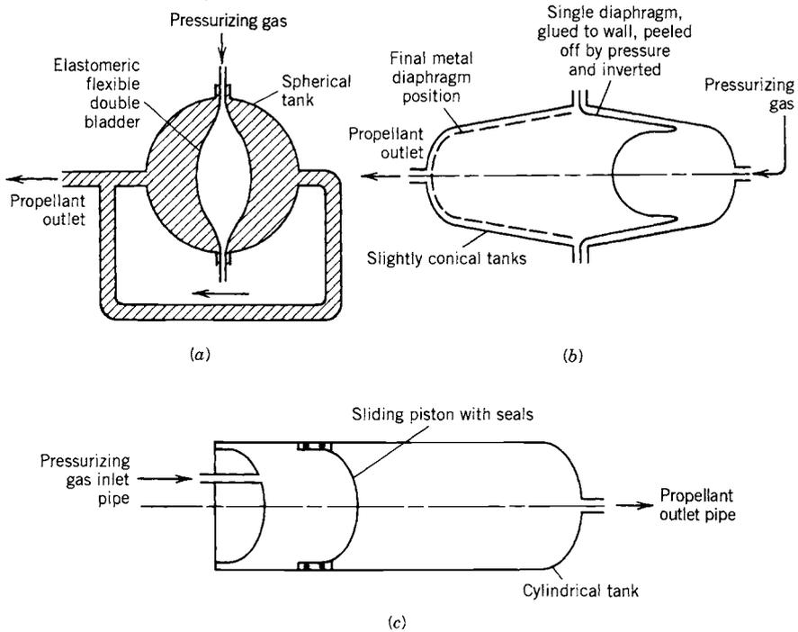
**FIGURE 6-7.** Three concepts of propellant tanks with positive expulsion: (a) inflatable dual bladder; (b) rolling, peeling diaphragm; (c) sliding piston. As the propellant volume expands or contracts with changes in ambient temperature, the piston or diaphragm will also move slightly and the ullage volume will change during storage.
