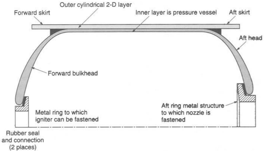
**FIGURE 14-4.** Simplified half-section of a typical design of a filament-wound composite material case. Elastomeric adhesives are shown in black. The outer layer reinforces the cylinder portion and provides attachment skirts. The thickness of the inner case increases at smaller diameter.
