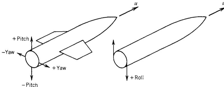
FIGURE 16-1. Moments applied to a flying vehicle.
