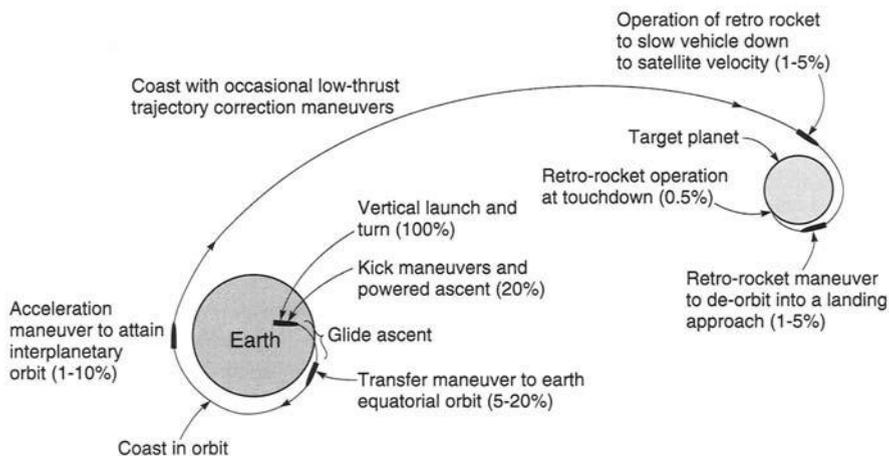
**FIGURE 4-10.** Schematic diagram of typical powered flight maneuvers during a hypothetical interplanetary mission with a landing. The numbers indicate typical thrust magnitudes of the maneuvers in percent of launch takeoff thrust. This is not drawn to scale. Heavy lines show powered flight segments.
