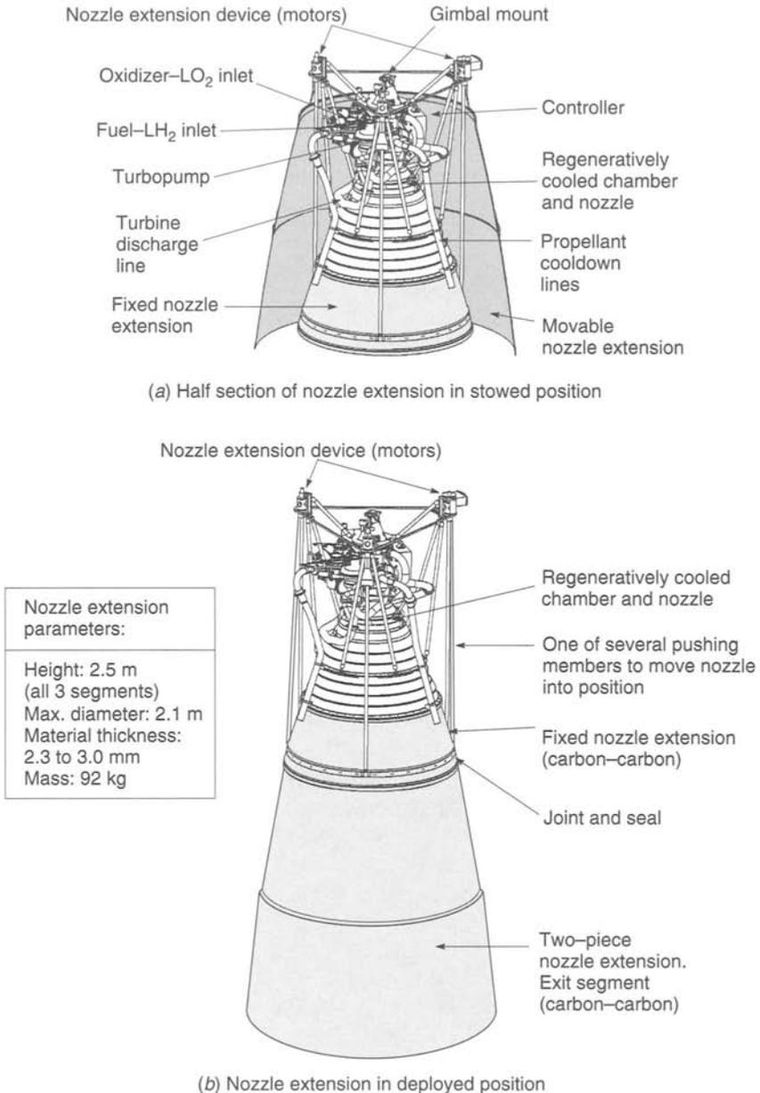
**FIGURE 8-19.** The RL-10B-2 rocket engine has an extendible nozzle cone or skirt, which is placed around the engine during the ascent of the Delta III launch vehicle. This extension is lowered into position by electromechanical devices after the launch vehicle has been separated from the upper stage at high altitude and before firing. (Courtesy of Pratt & Whitney, a division of United Technologies.)
