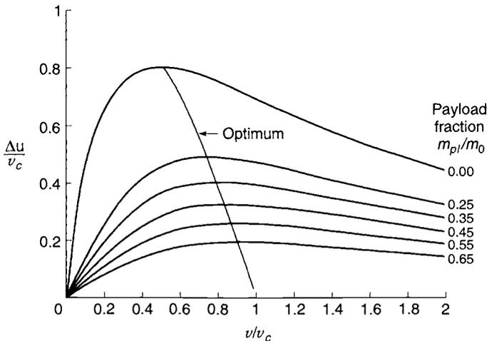
**FIGURE 19-3.** Normalized vehicle velocity increment as a function of normalized exhaust velocity for various payload fractions with zero inert mass of the propellant tank. The optima of each curve are connected by a line that represents Eq. 19-9.
