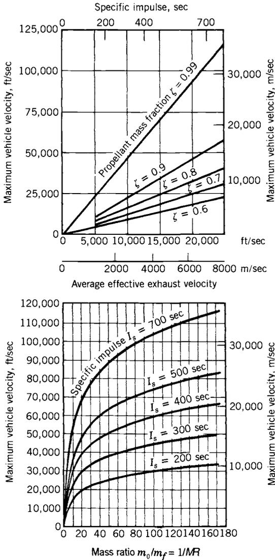
**FIGURE 4-2.** Maximum vehicle velocity in a gravitationless, drag-free space for different mass ratios and specific impulses (plot of Eq. 4-6). Single-state vehicles can have values of  $1/MR$  up to about 20 and multistage vehicles can exceed 200.
