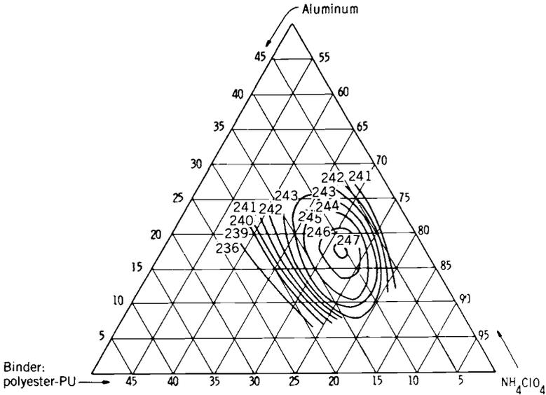
**FIGURE 12-4.** Composition diagram of calculated specific impulse for an ammonium perchlorate–aluminum–polyurethane (PU is a polyester binder) at standard conditions (1000 psi and expansion to 14.7 psi). The maximum value of specific impulse occurs at about 11% PU, 72% AP, and 17% Al. (Reproduced from Ref. 12-3 with permission of the American Chemical Society.)
