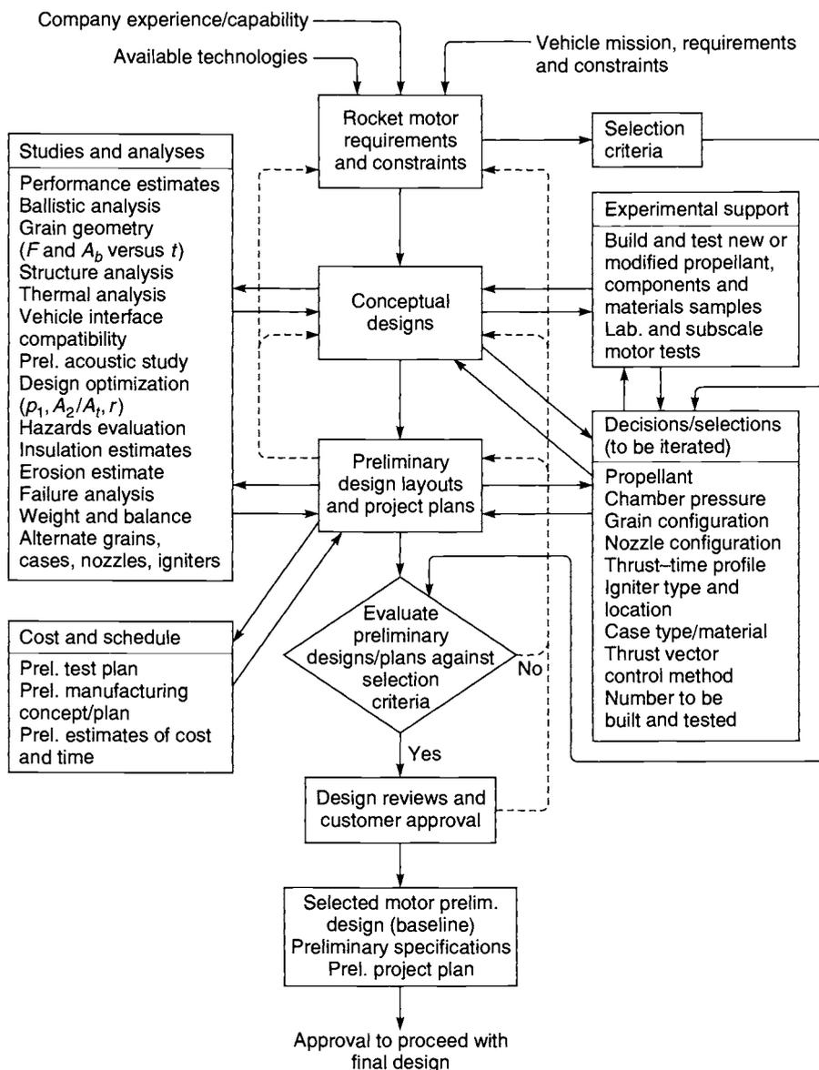
**FIGURE 14-17** Simplified diagram of one approach to the preliminary design activity sequences and interrelations. Dashed lines indicate some of the feedback paths. Some of the specific items listed here apply only to certain types of rocket motors.
