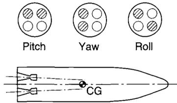
**FIGURE 16–10.** Differential throttling with four fixed-position thrust chambers can provide flight maneuvers. In this simple diagram the shaded nozzle exits indicate a throttled condition or reduced thrust. The larger forces from the unthrottled engines impose turning moments on the vehicle. For roll control the nozzles are slightly inclined and their individual thrust vectors do not go through the center of gravity of the vehicle.
