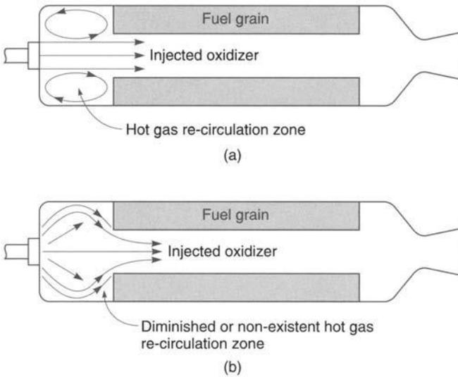
**FIGURE 15-13.** (a) Axial injection of oxidizer results in a strong hot gas flow recirculation zone at the fuel grain leading edge, producing stable combustion. (b) Conical injection of oxidizer can produce a weak or nonexistent hot gas flow recirculation zone at the fuel grain leading edge, resulting in unstable combustion.
