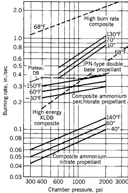
**FIGURE 11-6.** Plot of the burning rate versus chamber pressure for several typical solid rocket propellants, some at three different temperatures. A particular *double base* plateau propellant shows a constant burning rate over a fairly wide pressure range.
