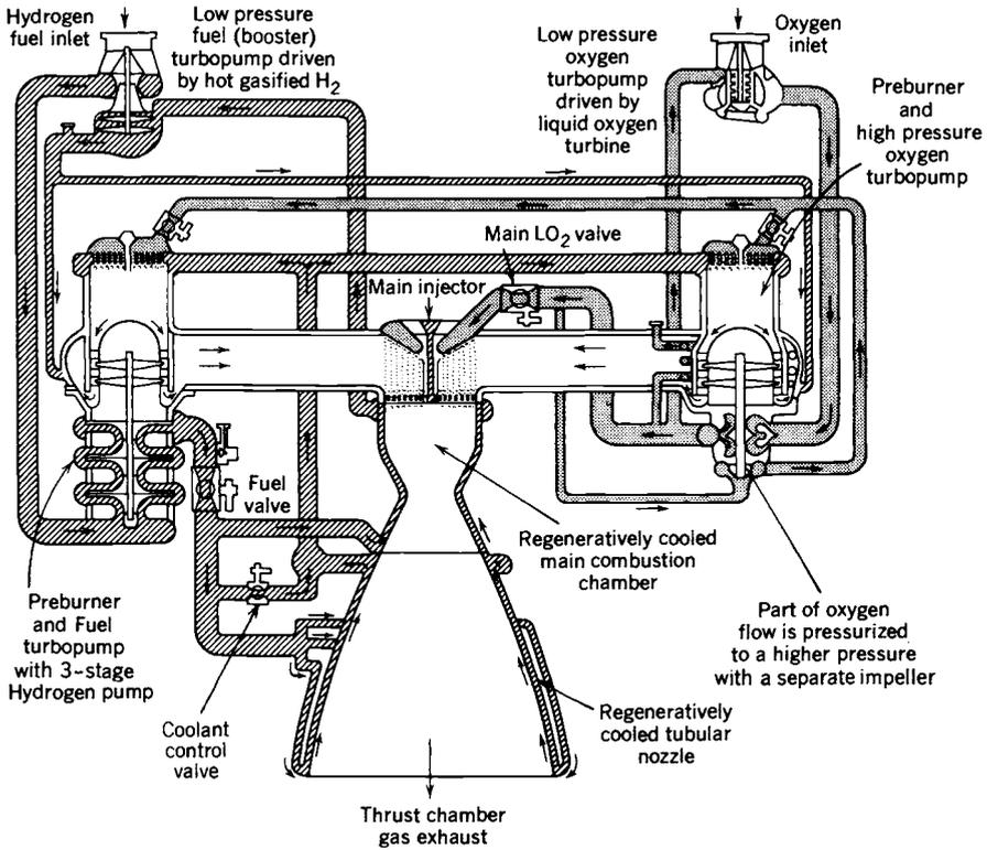
**FIGURE 6-12.** Flow diagram for the staged combustion cycle of the Space Shuttle Main Engine (SSME) using liquid oxygen and a liquid hydrogen fuel. (Courtesy of The Boeing Company, Rocketdyne Propulsion and Power.)
