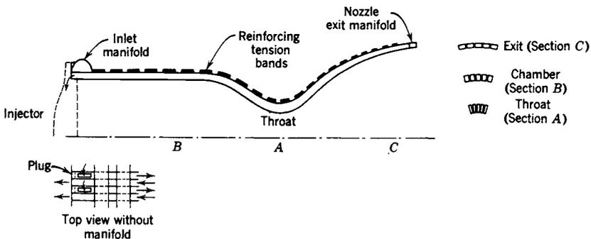
**FIGURE 8-9.** Diagram of a tubular cooling jacket. The tubes are bent to the chamber and nozzle contours; they are formed hydraulically to give a variable cross section to permit the same number of tubes at the throat and exit diameters. Coolant enters through the inlet manifold into every other tube and proceeds axially to the nozzle exit manifold, where it then enters the alternate tubes and returns axially to go directly to the injector.
