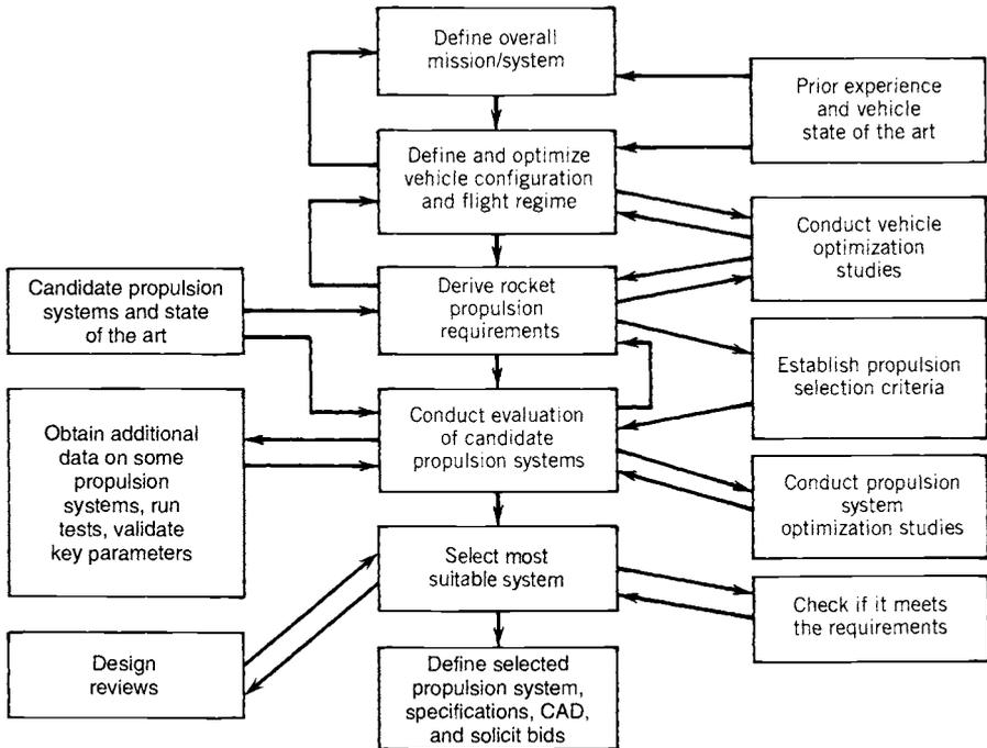
FIGURE 17-1. Idealized process for selecting propulsion systems.
