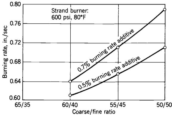
**FIGURE 12-8.** Typical effect of oxidizer (ammonium perchlorate) particle size mixture and burning rate additive on the burning rate of a composite propellant. (From NASA report SP-72262, Motor Propellant Development, July 1, 1967.)
