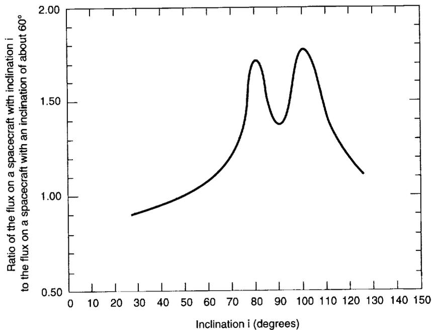
**FIGURE 4-4** Average collision probability variation with orbital inclination for cataloged LEO objects. SOURCE: National Aeronautics and Space Administration, based on data from the 1988 U.S. Space Command Catalog.
