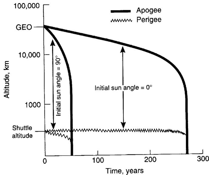
**FIGURE 7-4** Shuttle-launched LEO to GEO transfer stage lifetimes. Initial sun angle is the angle between the transfer stage's original orbit and the sun. SOURCE: Loftus et al., 1992.
