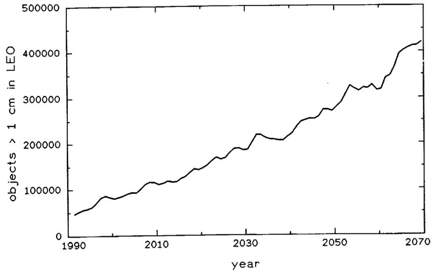
**FIGURE 8-2** Different model simulation of the future LEO space object population (constant launch rate and explosion rate at current level, no mitigation measures). SOURCE: National Aeronautics and Space Administration.
