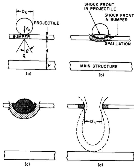
**FIGURE 6-1** Projectile interacting with a spaced shield. (a) impact onto a thin bumper plate, (b) penetration, (c) subsequent formation of a spallation cone, and (d) loading transmitted by the cone to the catcher. SOURCE: Riney, 1970.
