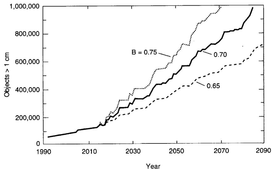
**FIGURE 8-5** Effect of assumed mass distribution of collision fragments ( $B$ ) on prediction of future population of objects larger than 1 cm. The three scenarios are the result of Monte Carlo simulations run with the same stochastic numbers but with different assumed mass distributions of collision fragments. In all scenarios, the basic population (launched objects plus collision fragments) increases by 3,000 objects >1 cm per year. SOURCE: Eichler, 1993.
