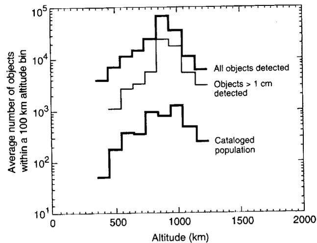
**FIGURE 3-8** Estimate of LEO mid-sized orbital debris population from Haystack radar sampling (90 degrees, 547.6 hours), compared to the U.S. Space Command population of cataloged objects. SOURCE: National Aeronautics and Space Administration.
