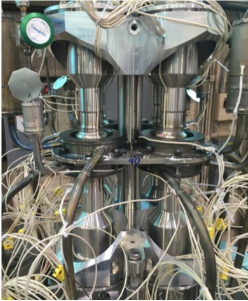
Figure 3. Balance of Plant hardware showing 8 sodium heat pipes attached to a conduction plate that supplies heat to 2 Stirling engines and 6 Stirling thermal simulators.
