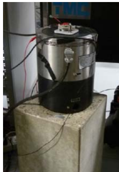
(a) EPFL SAMLAB's magnetic shaker table.
