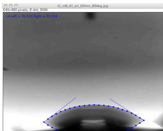
(a) EMI - BF_4 on MVD B, in air at 80^\circ C
