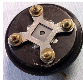
(c) Test sample mounted on test assembly
