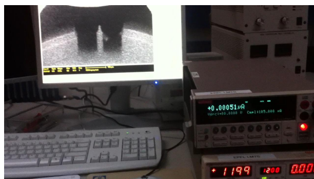
(a) Emitter = 0V, Extractor = 1200V, Shield = 0V
