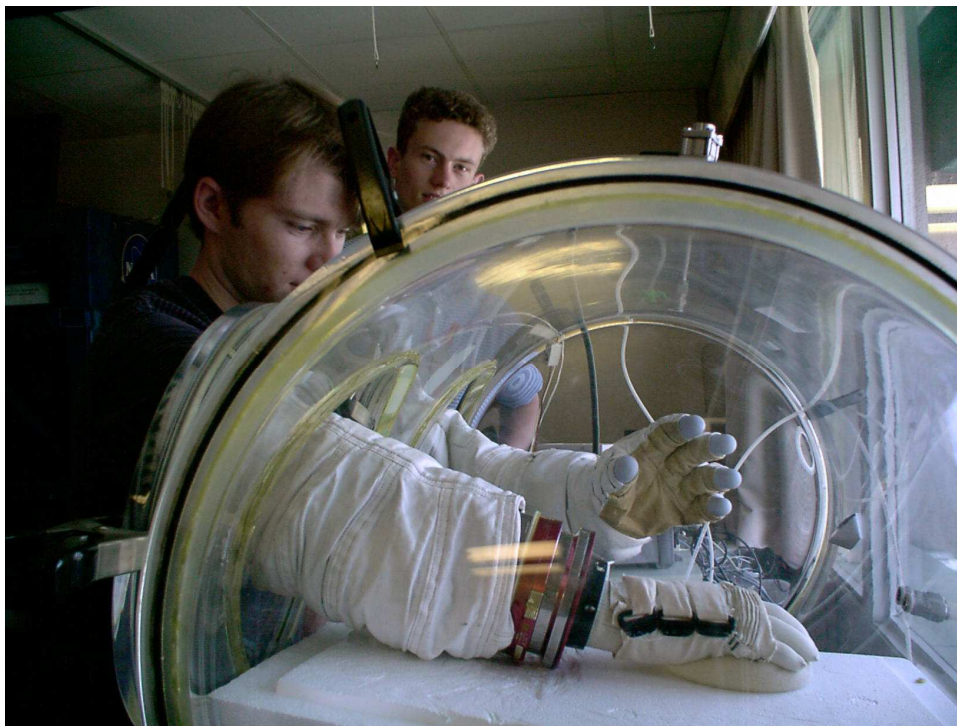
Fig.1: Qualitative comparison of MCP and shuttle gloves in a hypobaric chamber
