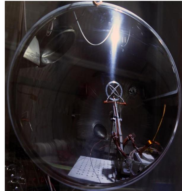
**Magnetoshell installed in chamber.** *Shown are two in-chamber power supplies (potted), low-inductance stripline, G-10 mount.*
