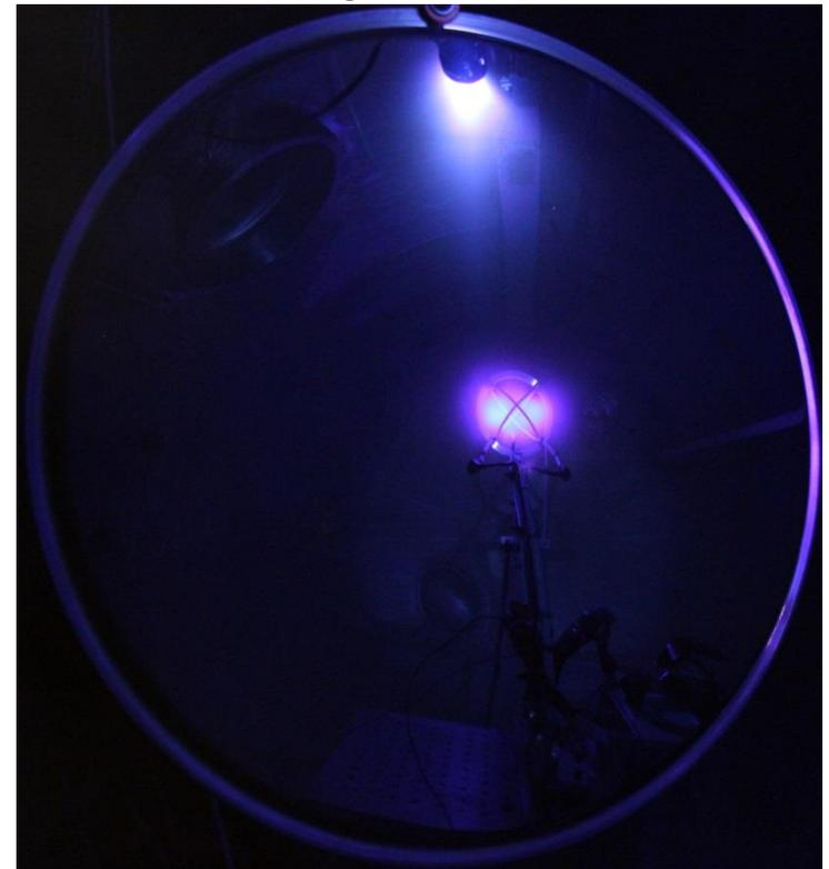
**Magnetoshell operating with internal gas feed and intercepting an accelerated neutral and plasma jet.** Shown is 50 sccm internal feed, 3 Joule RF, and 1 ms MPD discharge at 1.2 kV following a 20 ms neutral puff.
