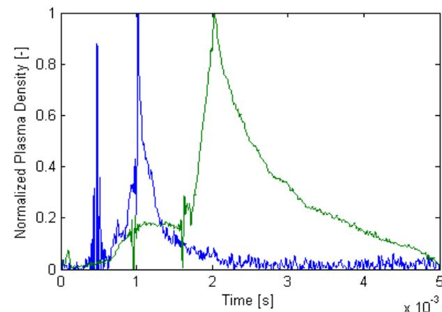
MPD downstream plasma density with and without a neutral pre-gas as blue and green, respectively.
