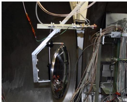
MPD mounted in the MSNW vacuum facility. **Shown is the MPD with integrated puff valve, spherical mirror, and in the background, the 'waterfall' power feed lines.**
