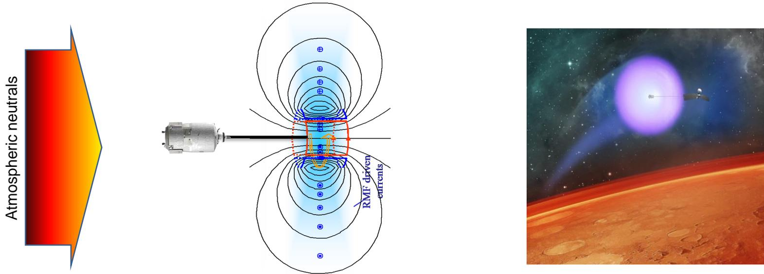
1. A spacecraft deploys Magnetoshell hardware on a 50 meter tether
