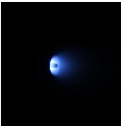
Pulsed MPD operating with an argon propellant and 2 ms discharge.
