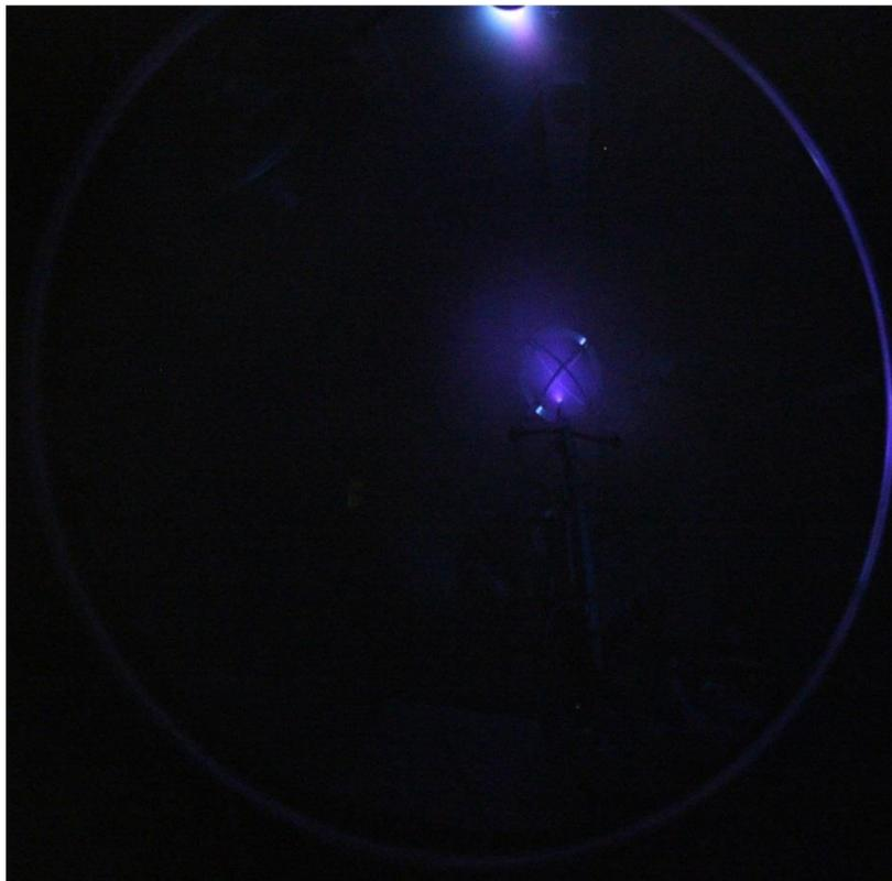
**Magnetoshell operating with internal gas feed and intercepting only MPD plasma.** Shown is 50 sccm internal feed, 3 Joule RF, and 1 ms MPD discharge at 1.2 kV and 1 ms delay.
