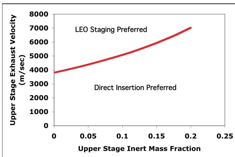
Figure 1. Delivered Payload Break-Even between LEO Staging and Direct Insertion to Destination
