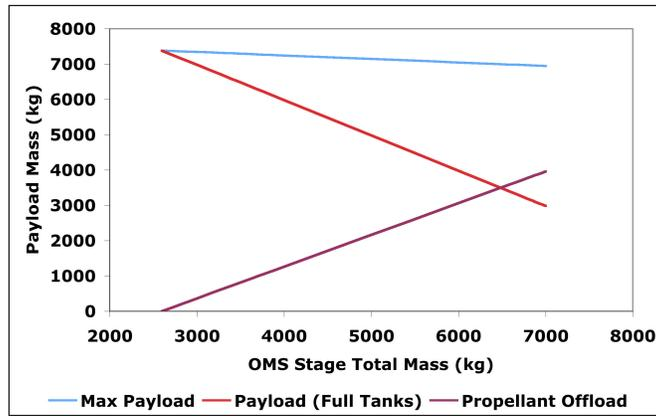
Figure 2. Effect of Orbital Maneuvering Stage Mass on Delivered Payload
