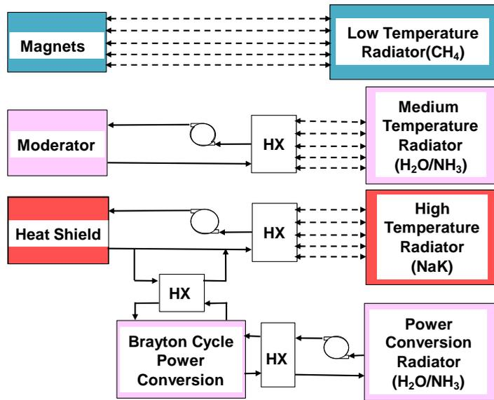
Four double sided, radiator systems constructed of composite materials keep this FFRE design within its thermal limits by rejecting over 700 MW to space. These radiators total over 56000 ft<sup>2</sup> and would be folded to fit within a Heavy Lift Launch Vehicle payload shroud. The masses, including MGA, are shown in the accompanying table and total a massive 64 mT including MGA.
