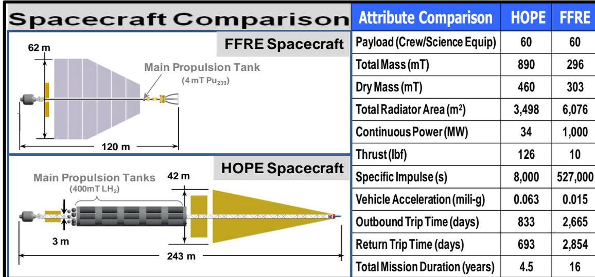
stages. This hydrogen would have to be maintained in a cryogenic condition throughout the mission, a formidable task. These immense hydrogen tanks would be shed as the propellant is consumed during each engine burn. Consequently for a subsequent mission, at least five Heavy Lift flights would be needed just for replenishment of the needed hydrogen and for new tanks.
