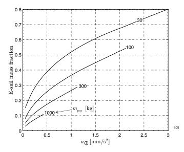
**Fig. 3.** E-sail mass fraction as a function of  $a_{\oplus}$  and  $m_{\text{pay}}$ .
