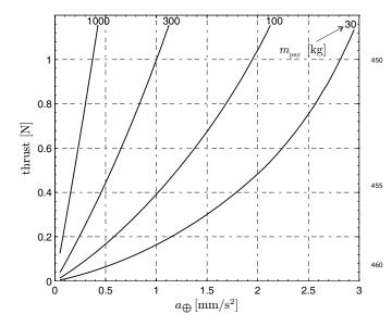
**Fig. 6.** E-sail thrust at 1 au as a function of  $a_{\oplus}$  and  $m_{\text{pay}}$ .
