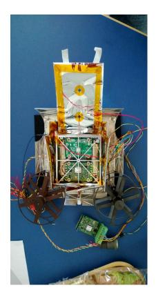
• Remote Unit *m*=0.56 kg (CG version dry), allowed solar distance range 0.9-4 au
