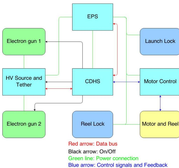
Fig. 1: Block diagram depicting the data and power interactions between PL parts, CDHS and EPS.
