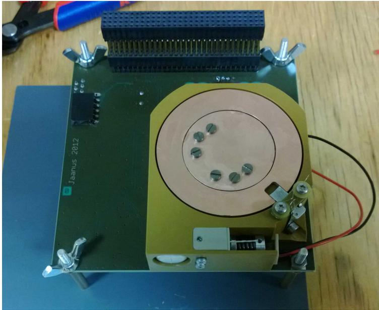
Fig. 11: Motor board fully assembled.
