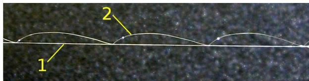
(a) Photograph of tether. Labels: (1) Basewire, (2) Loop wire. Distance between bonds is 10 mm.
