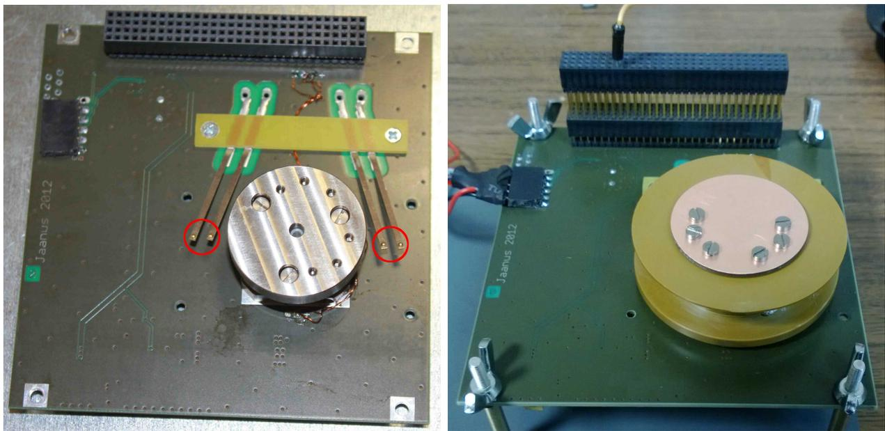
(a) Reel motor attached on the circuit board. Shown circled are the four slip ring contacts.
