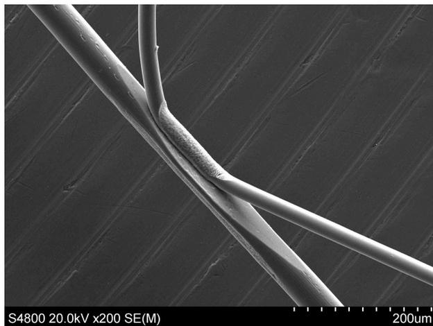
(b) Scanning Electron Microscope (SEM) image of an ultrasonic wire-to-wire bond.
