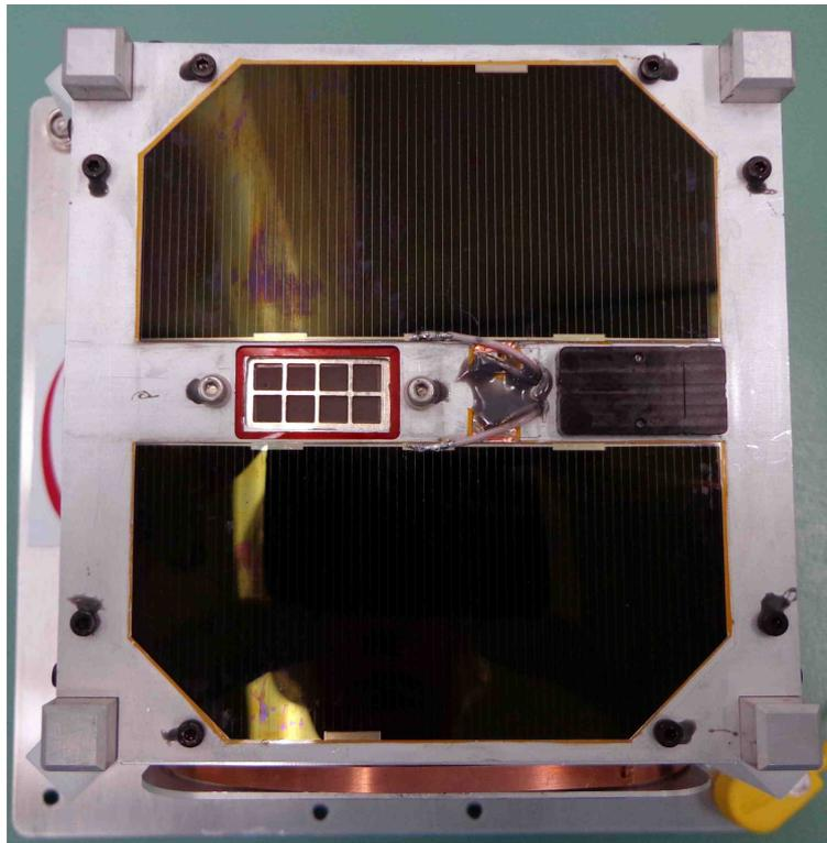
Fig. 16: Electron gun attached on satellite side panel.
