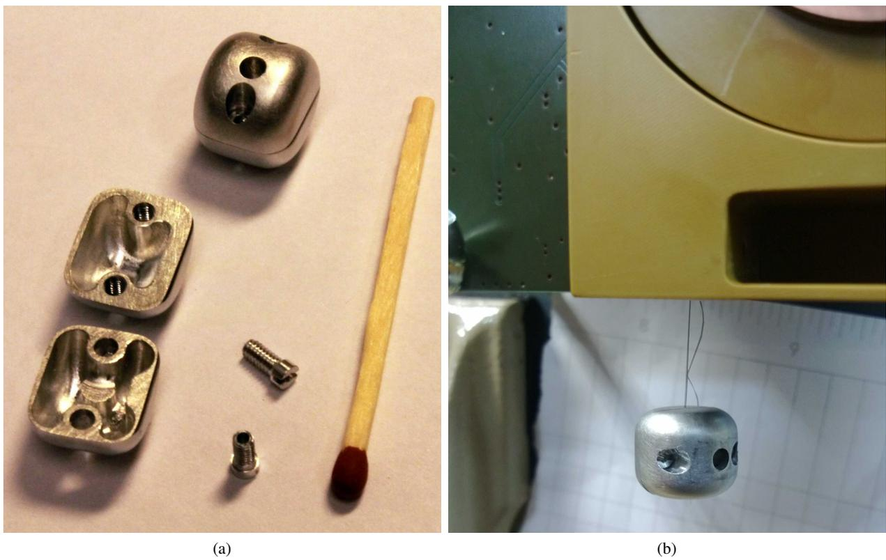
Fig. 9: (a) Assembled and stripped down view of end mass. (b) End mass hanging from the tether during PL assembly. Tether enhanced digitally for visibility. Notice the middle hole for the launch lock pin.
