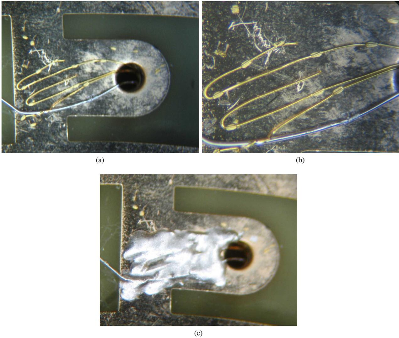
Fig. 8: Slip ring bond. (a) Basewire and three gold wires bonded on slip ring. (b) Closeup of the same bonds. (c) All bonds covered with conducting glue.
