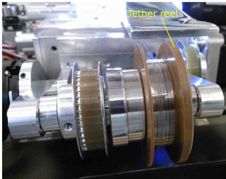
Fig. 4: Tether being manufactured on the reel at UH in January 15th, 2013.
