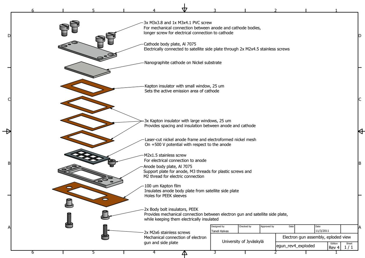
Fig. 14: Exploded view of electron gun.
