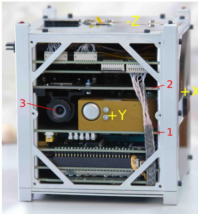
Fig. 2: Assembled satellite with side panels removed. Labels: (1) Motor board, (2) HV board, (3) onboard camera. The yellow labels denote the directions of X, Y and Z axes of the satellite's coordinate system.
