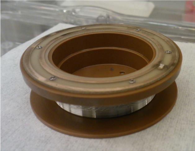
(b) Slip ring attached on reel, tether bonded and reeled.
