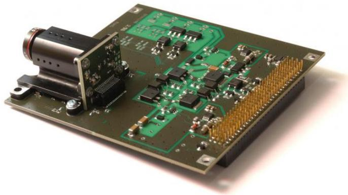
Fig. 12: High voltage board. The large black block is the onboard camera.
