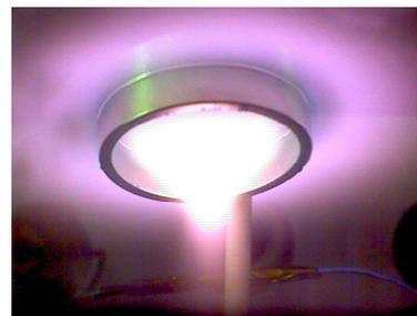
Figure 7. Magnetic quadrupole confinement of ion plasma.
