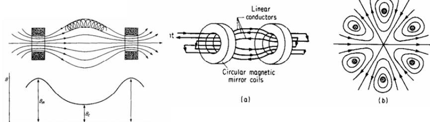
Figure 6. Magnetic confinement of fission fragments in a magnetic mirror. Stronger field on one end reflects fragments, weaker field on nozzle transmits particles. Wall fields are strengthened by multipole fields such as this hexapole current arrangement.
