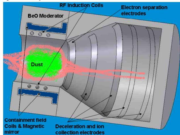
Figure 2. Schematic of proposed Fission Fragment Rocket. Fissile dusty plasma fuel is confined to dust chamber, where RF induction coils heat the plasma. Fission fragments are collimated by the magnetic field either to collection electrodes for power, or exit the reactor for thrust.
