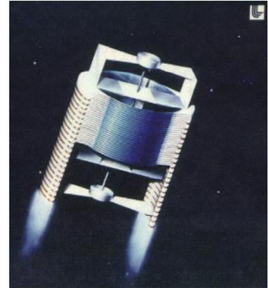
Figure 1. Fission fragment concept as proposed by Dr. George Chapline. The reactor consists of thin carbon filaments coated with nuclear fuel rotated at high speed through the core. Courtesy of LLNL.
