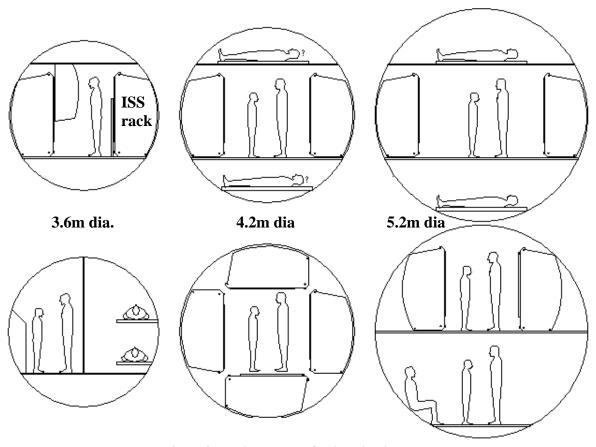
Figure 3. Possible layouts for 3 cabin diameters
