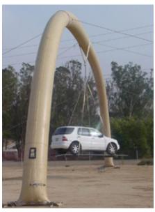
Figure 6. Airbeam supporting a car
