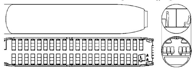
Figure 5. A 3.6x17m cabin compared to a 737-600 cabin
