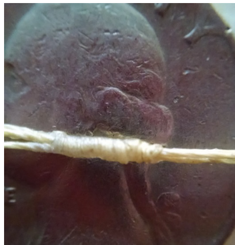
Figure 63: Kevlar tied with Kevlar. Quarter background for scale.
