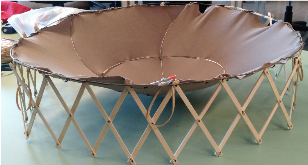
Figure 25: An early prototype of the drum support using a collapsible scissor frame.
