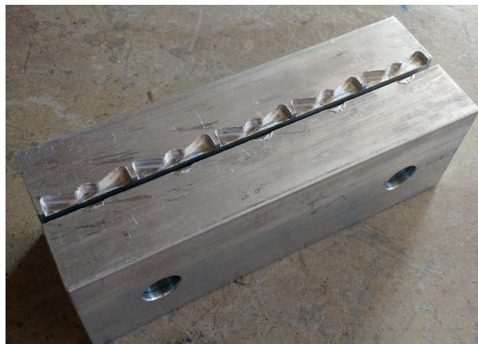
Figure 41: Soft jaw fixture used to face sliders to correct height
