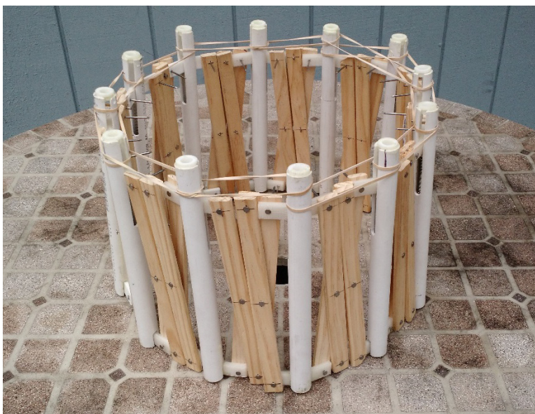
Figure 27: Drum prototype in the stowed configuration, scaled up with 1cm = 1in.
