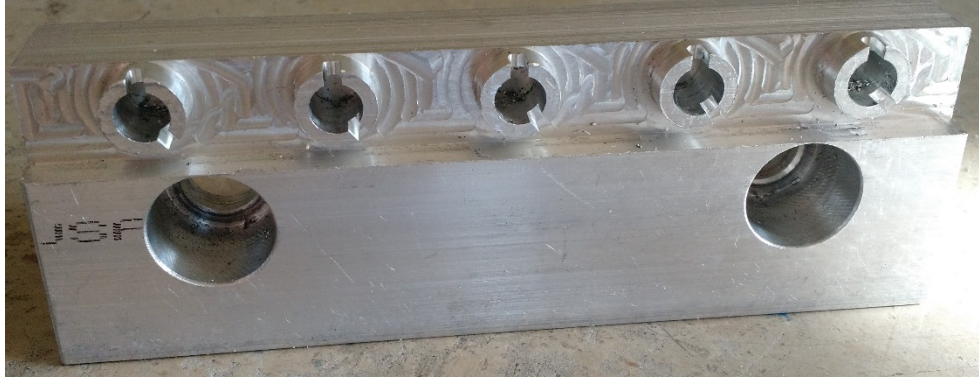
Figure 49: Fixture designed with deep bores for support cores. Two locating slots assist in aligning stock
