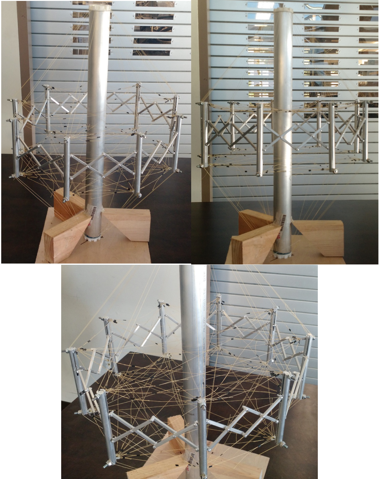
Figure 67: The final assembled design with placebo mast and Kevlar tension ties connecting the truss to the mast.
