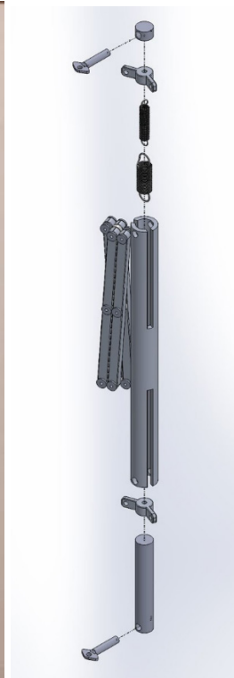
Figure 59: Left: Internal look at a vertex when truss is deployed (not to scale) Right: SolidWorks assembly of vertex and components..
