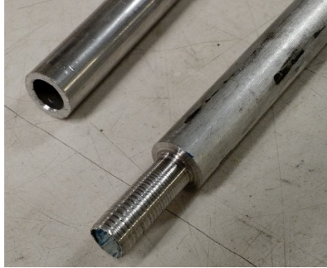
Figure 47: Stock milled down and used as support cores for vertices
