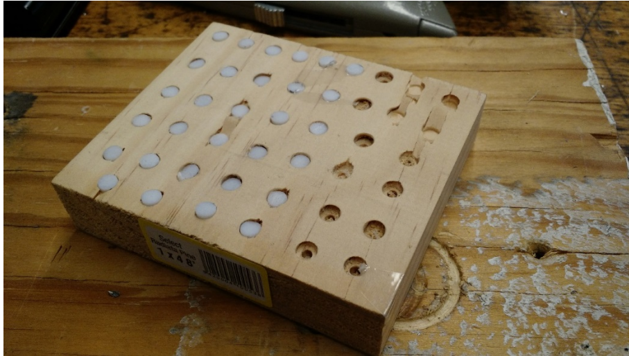
Figure 55: Jig used to drill holes in spacers
