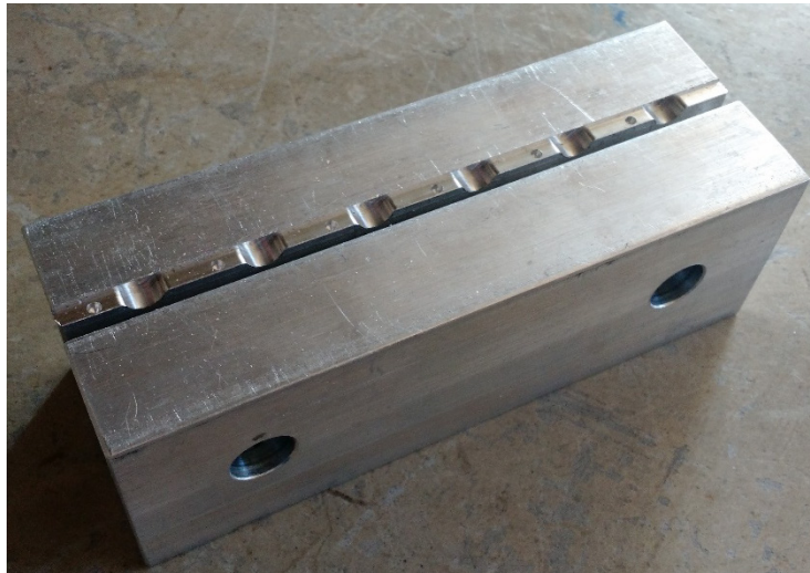
Figure 42: Fixture used to drill holes in winglets of sliders.
