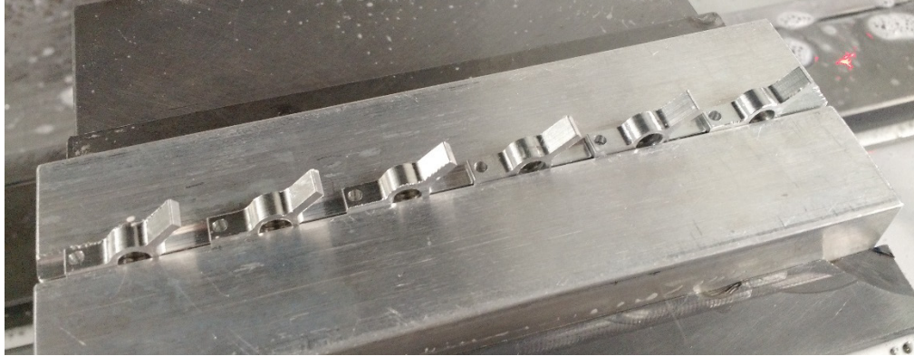
Figure 44: Sliders with holes after completion of CNC drilling operation
