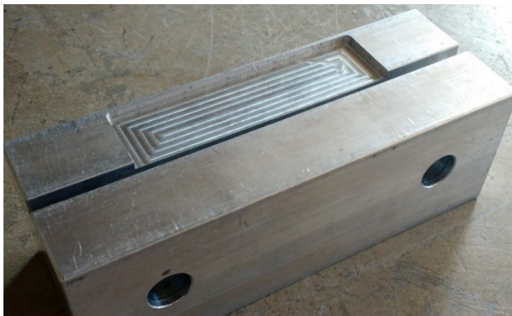
Figure 54: Fixture used to face down testing struts to the correct thickness
