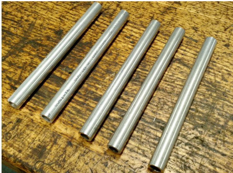
Figure 45: Tube stock cut to design length of vertices
