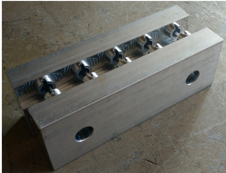
Figure 46: Fixture used to mill slots of vertices
