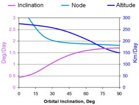
Figure 5: EDDE Orbit Transfer Performance
