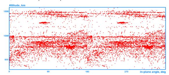
Figure 1: Tracked Objects Crossing the Orbital Plane of a Spacecraft in LEO
