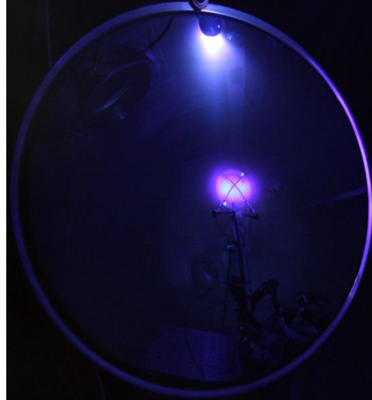
Figure 37. Magnetoshell operating with internal gas feed and intercepting an accelerated neutral and plasma jet. Shown is 50 sccm internal feed, 3 Joule RF, and 1 ms MPD discharge at 1.2 kV following a 20 ms neutral puff. Shot #20198
