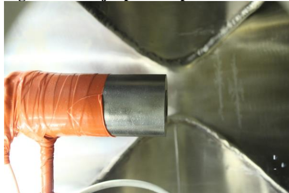
Figure 27. Arcjet mounted in the 'Junior' test facility.
