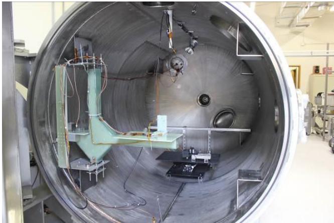
Figure 20. 2 m MSNW vacuum chamber with dielectric, asymmetric torsional thrust stand.
