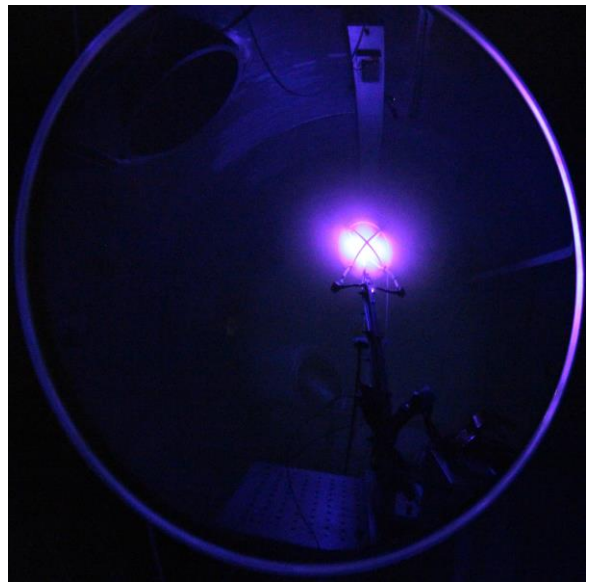
Figure 35. Magnetoshell operating with internal gas field and intercepting a partially ionized jet Shown is 50 sccm internal feed, 3 Joule RF, and 20 ms neutral gas puff. Shot #20178
