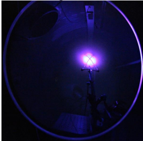
Figure 2. Magnetoshell operating with internal gas field and intercepting a partially ionized jet.
