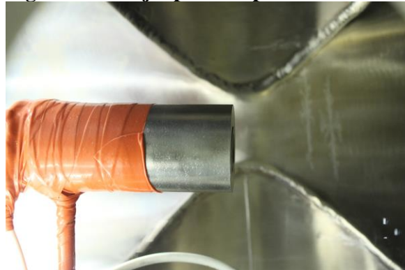
Figure 27. Arcjet mounted in the 'Junior' test facility.
