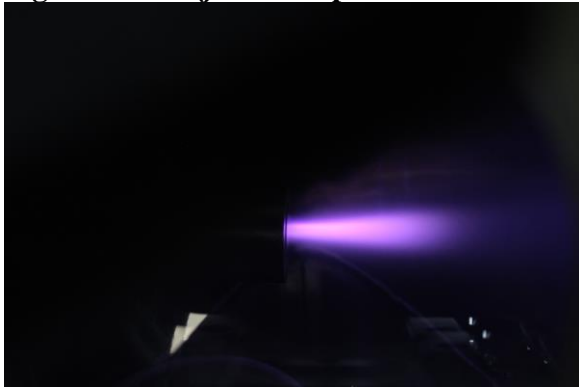
Figure 26. Arcjet pulsed operation – 100 ms.
