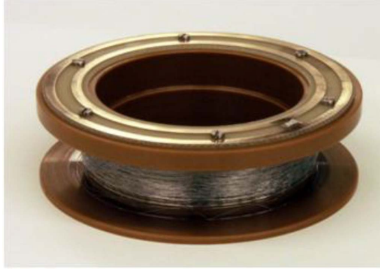
(b) 15 m of tether on the flight reel.
