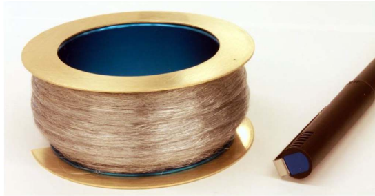
(c) 1 km of tether on the output spool.
