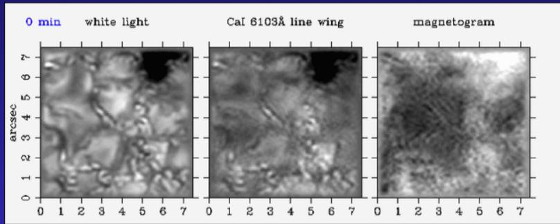
Phase-diverse speckle imaging uses in-focus and out-of-focus image sequences to completely remove the aberrations due to the Earth's atmosphere and the telescope over a field of view that is much larger than the isoplanatic patch.
