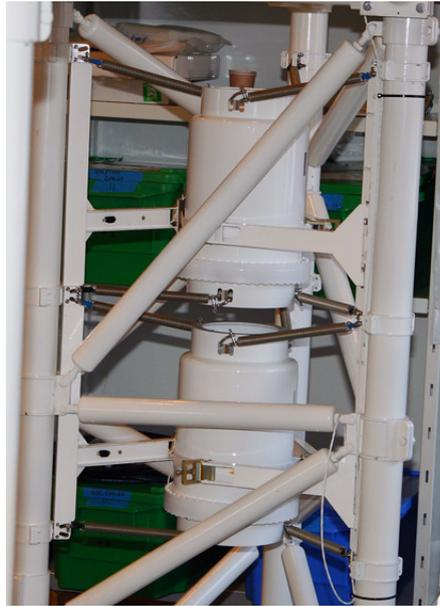
Figure 4.10: The 2 pressurized vessels of the Data Storage Subsystem.
