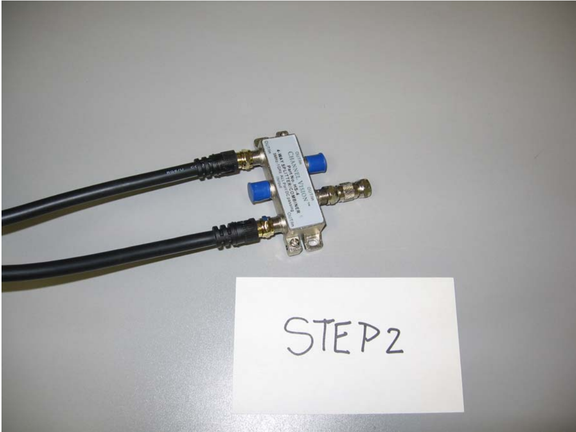
Figure 7. Step 2: Attach splitter to cables
