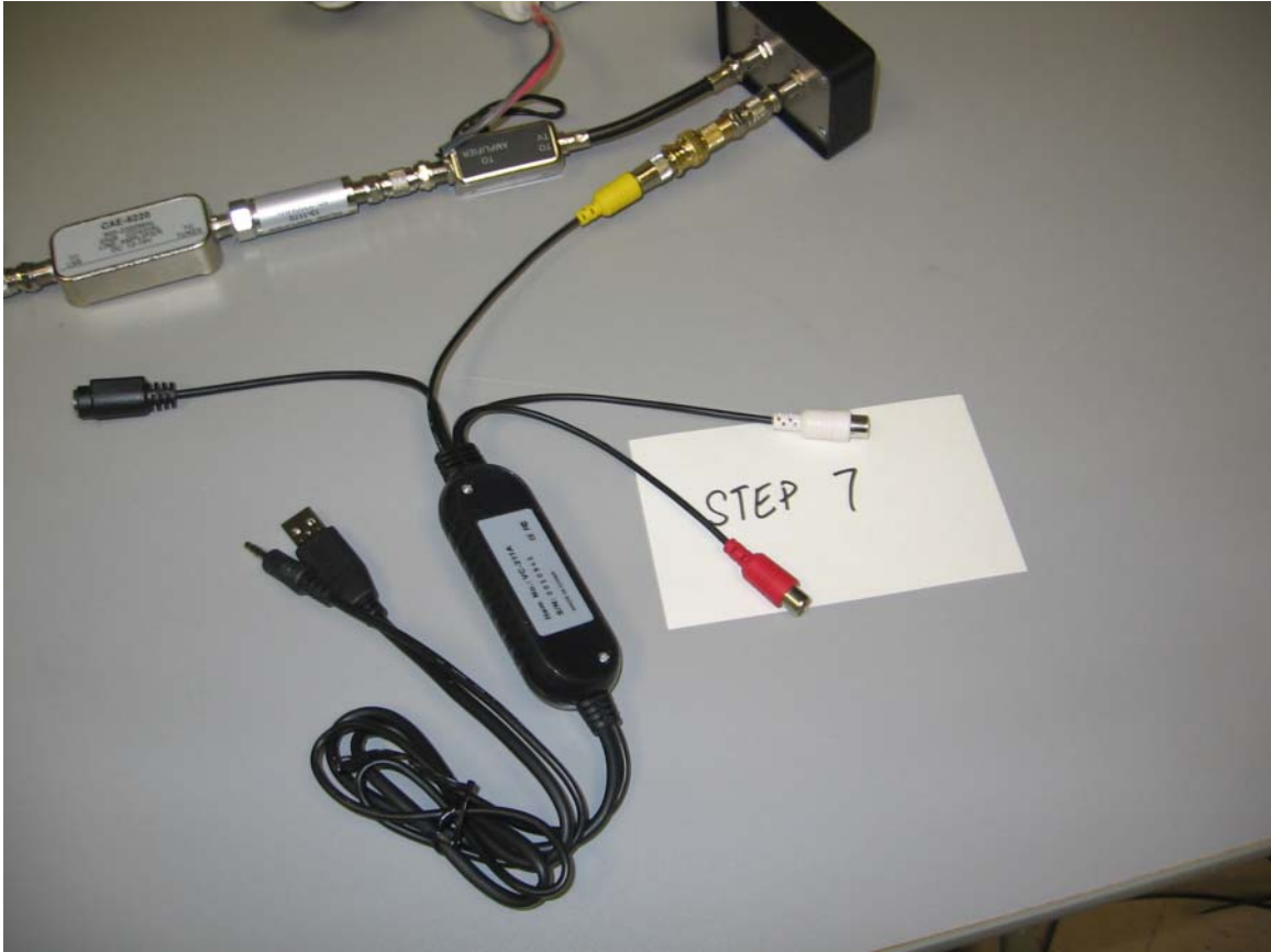
Figure 12. Step 7: Attach the video frame grabber. The USB end of the frame grabber will go into the computer.
