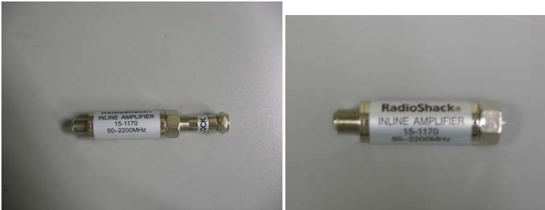
Figure 8. Remove DC block from inline amplifier. You will need to remove the plastic covering and unscrew.
