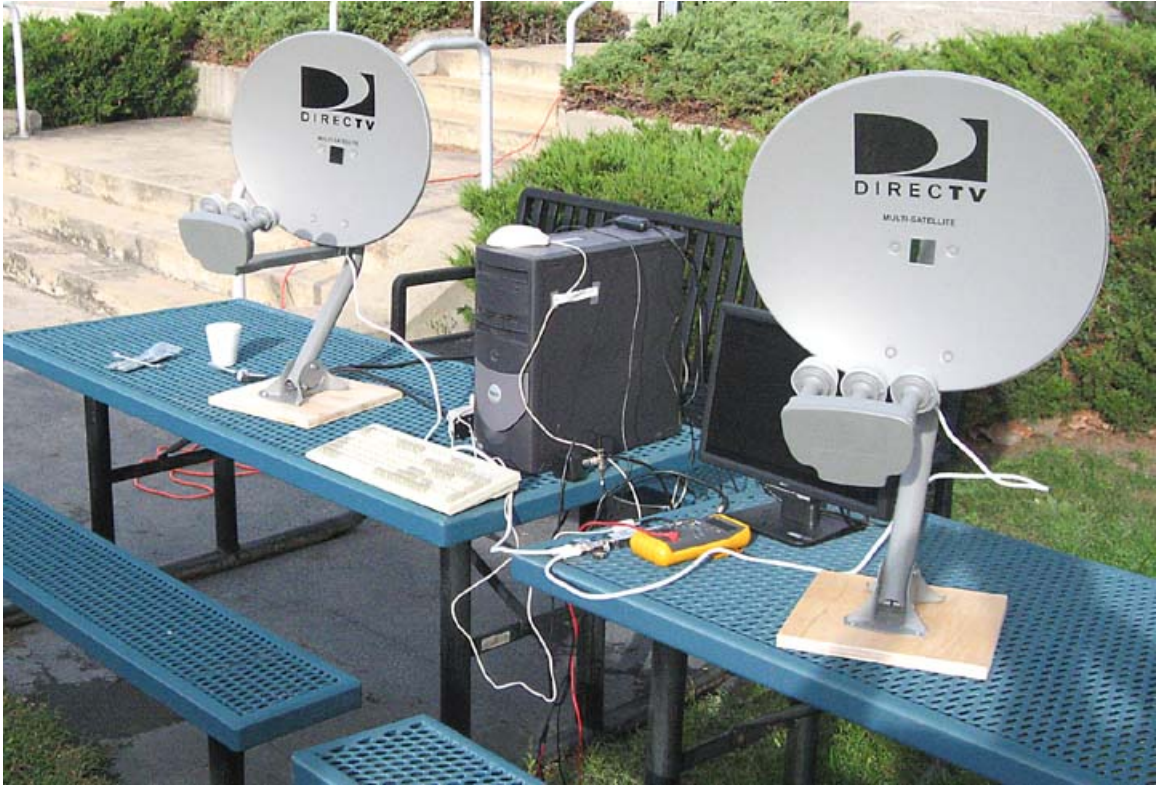
Figure 5. Set-up to observe the Sun.
