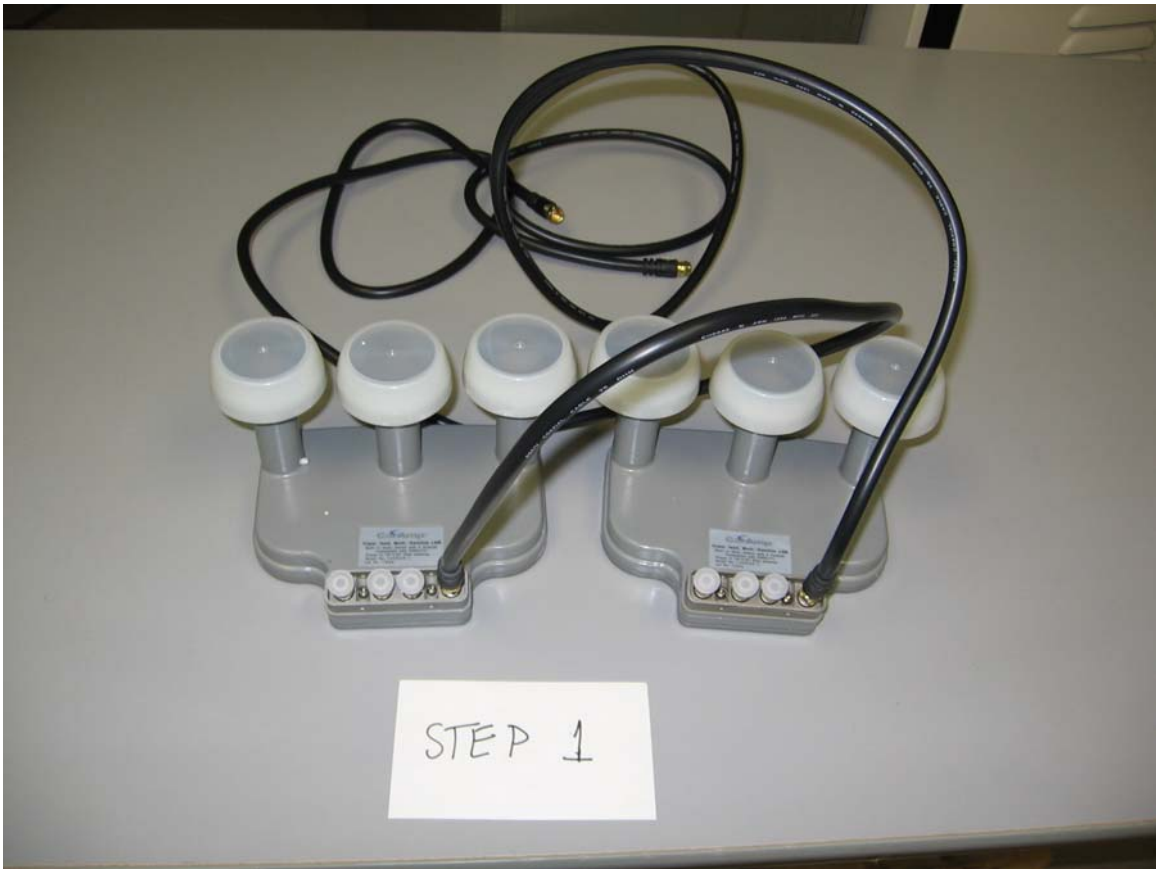
Figure 6. Step 1: Attach cables to LNBs
