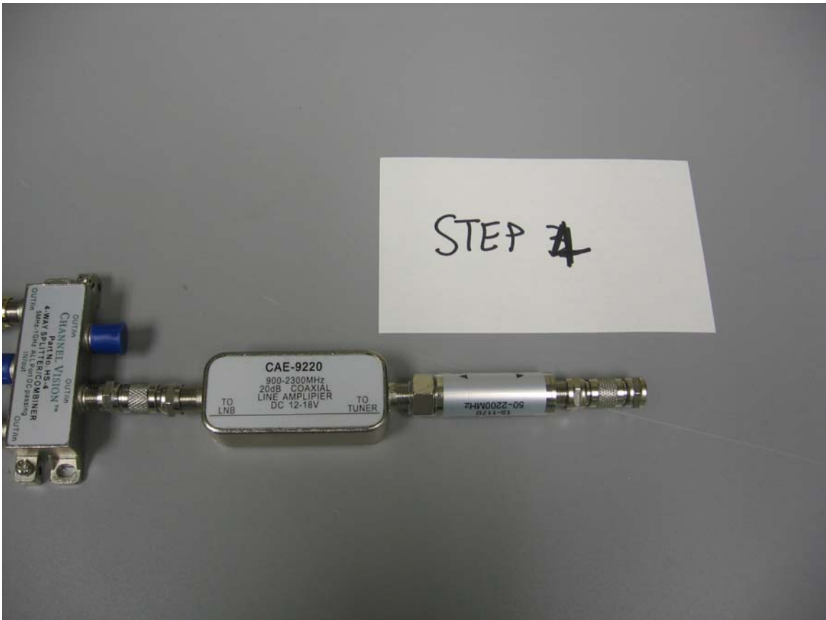
Figure 9. Step 4: Attach the inline amplifier and another “male to male” connector.
