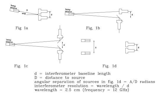
Figure 1. Suggested set—up for laboratory demonstrations using compact arrangement of 2 feeds for a single baseline
