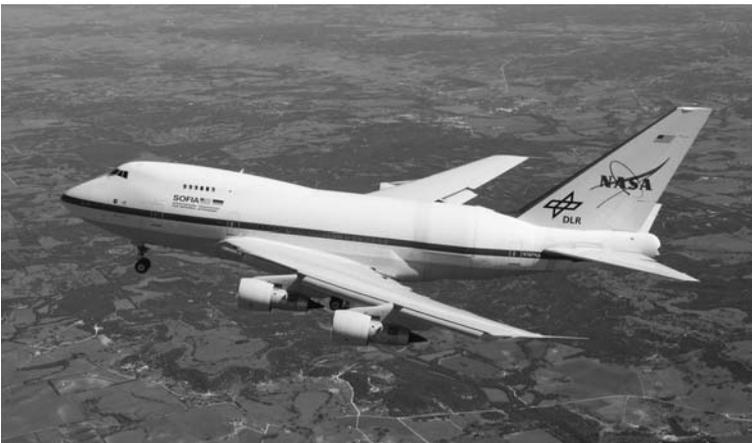
**Fig. 7.12** The SOFIA facility will fly at about 12 km altitude, above most of the water in the earth’s atmosphere. This will allow measurements in the sub-mm and far infrared range. The modified 747SP airplane contains a 2.5 m optical telescope. This is a joint project of NASA and the German Space Agency, DLR. The first test flights are now taking place
