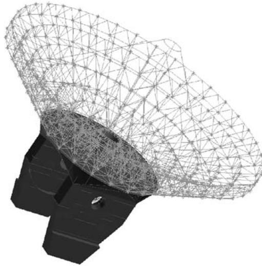
**Fig. 2.9** IRAM 30-m telescope illustrating the connection of the BUS network to the roof (membrane) of the yoke. The BUS is a homologous design requiring the membrane connection to the yoke (see also Fig. 6.6) [From Bremer & Peñalver (2002), Courtesy SPIE].
