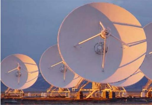
**Fig. 5.7** Asymmetric solar illumination of parabolic reflectors of the VLA array (NM, USA) [Image Courtesy of NRAO/AUI/NSF].
