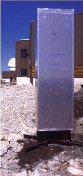
**Fig. 11.2** Model of a fork arm ('chimney' experiment) for the study of different types of insulation. The measurements were made on Plateau de Bure under representative meteorological conditions.
