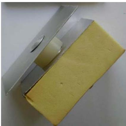
**Fig. 11.15** IRAM 15-m telescopes. The applied thermal protection consists of insulation (5 cm), aluminium foil, an air gap (2 cm) and a radiation shield (Al-plate) that is the outer surface. The supports of the radiation shield are plastic spacers with screws.
