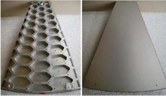
**Fig. 2.13.b** Machined Aluminium panel (IRAM 15-m telescope); left: rear side with hexagonal support boxes, right: front surface. The panel is machined from a solid aluminium plate [Courtesy IRAM, France].
