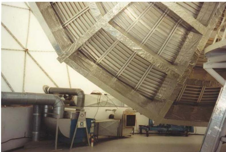
**Fig. 3.5** FCRAO telescope (Amherst, USA) inside the radome. The telescope is covered in aluminium foil. Note the ventilator at the periphery of the radome [Courtesy F.P. Schloerb, FCRAO, USA].
