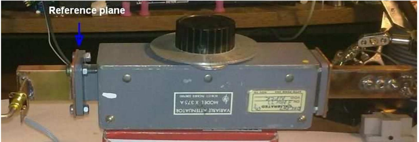
Fig. 11. Waveguide noise source: central part – attenuator ~ 20 dB, right part – solid state noise generator, left part – LNA under test.
