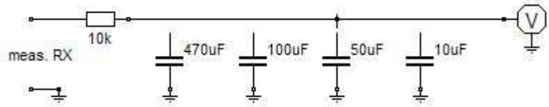
Fig. 6. Averaging RC circuit at the measuring receiver output.
