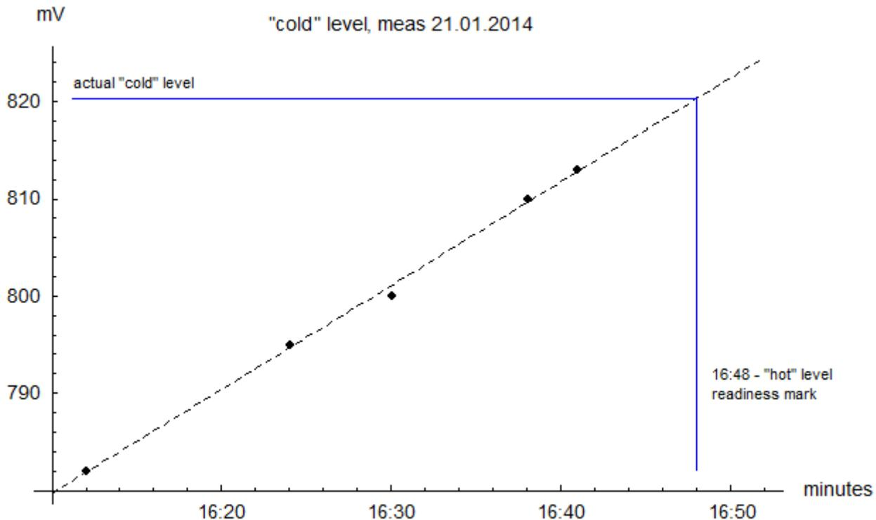
2. Next, I interpolated the dots; interpolation curve is a simple straight line usually, but some assurance is needed about and a plot showing the curve and readouts is very useful for. The line corresponds to the gain drift; and this line can be extrapolated further, so, one can predict a future levels of "cold" readouts if so could be done.
