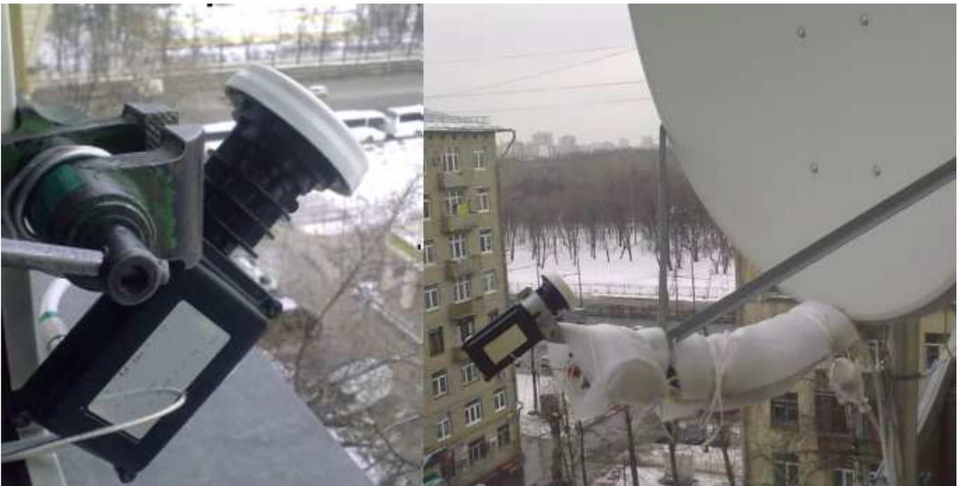
Fig. 10. LNA with permanently attached horn made from old Sat converter "Cambridge", circular polarization.
