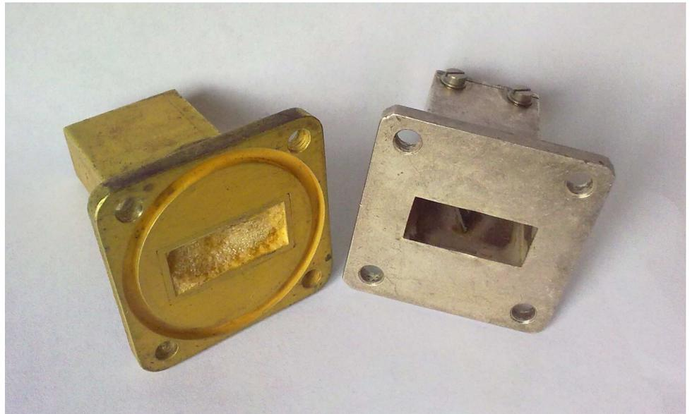
Fig. 4. Dummy loads, waveguide size WR90.
