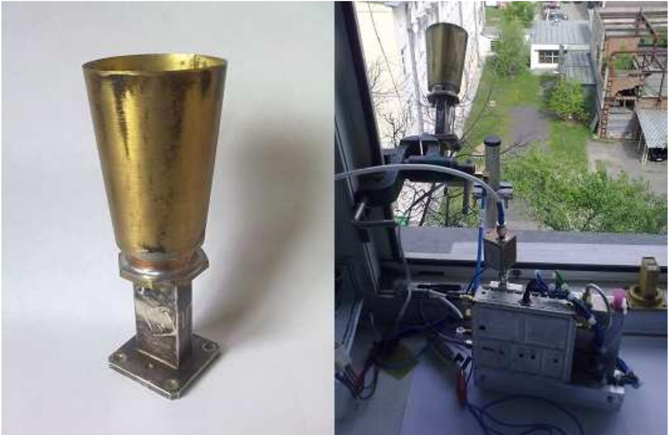
Fig. 3. 10 GHz Skobelev horn for NF measurements.
