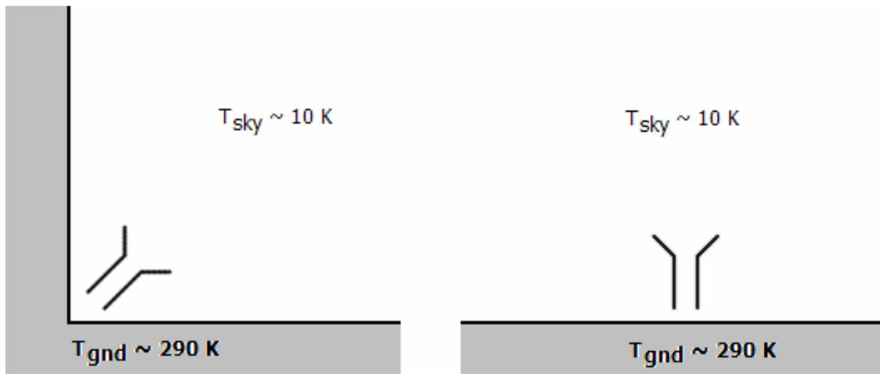
Fig. 2. Two possible situations in Cold Horn measurements: left – the horn placed near a wall with ambient temperature about 290 K, right – the horn looking to zenith, no any wall present. I assumed the Sky has a noise temperature about 10 K at 10 GHz.
