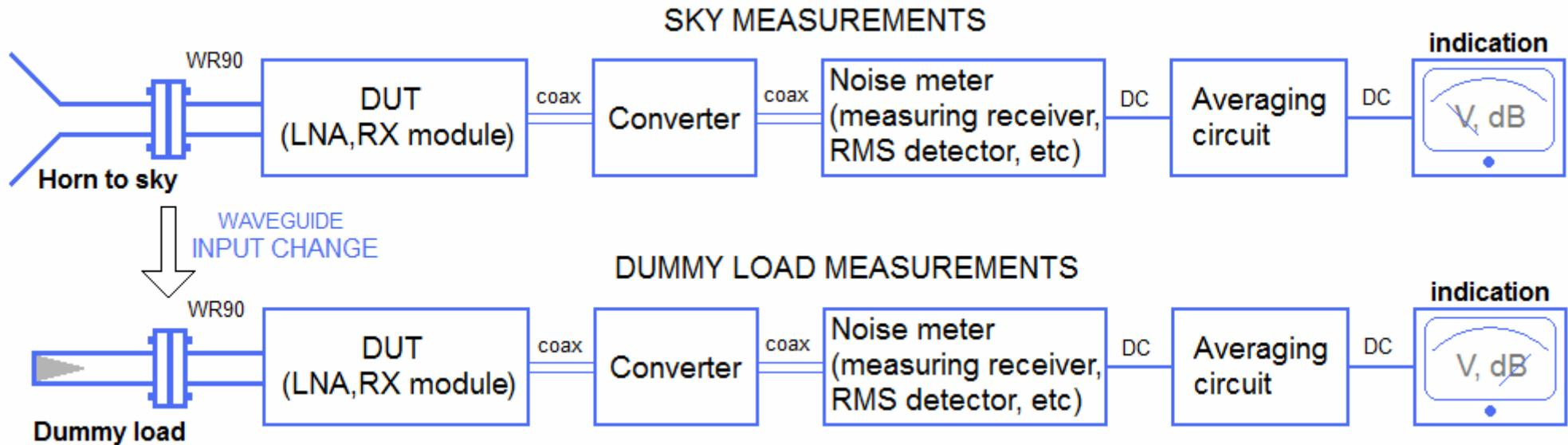
Fig. 5. Schematic (block diagrams) for Noise Figure measurements by Cold Horn.
