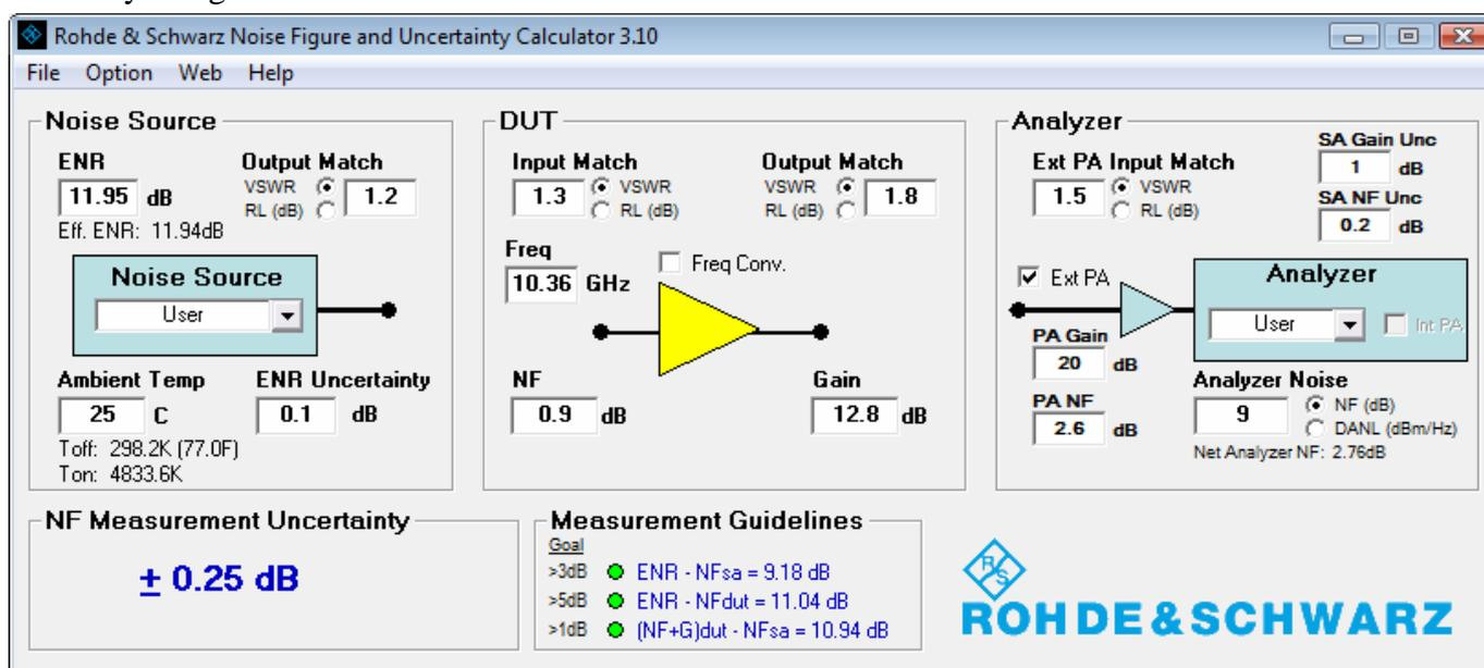
Fig. 1. The estimation of NF uncertainty at 10 GHz for typical LNA (NF=0.9 dB, Gain up to 13 dB and moderate VSWR at input and output. Noise head is characterized by ENR value with typical uncertainty  $\delta ENR=0.1$  dB, and output VSWR or reflection coefficient.
