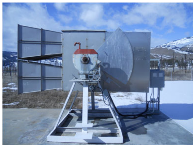
Figure 8. Calibration Horn system seen from the East. Two identical horns are mounted piggyback. The electronics is housed in the casing on the back of the horns. Antenna driving is manual, using the large declination scale for pointing. The upper horn is the one currently used.
