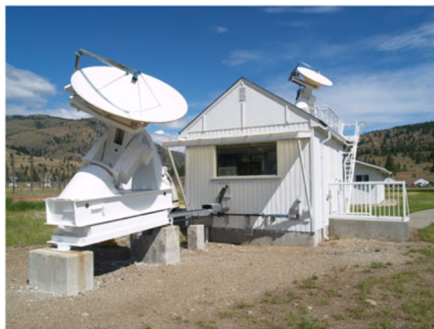
Figure 3. The flux monitors. Flux Monitor 1, the secondary instrument is in the foreground; Flux Monitor 2, the primary instrument is in the background, on the tower.
