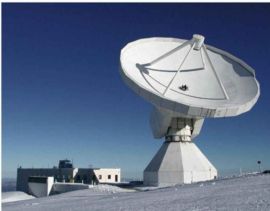
The 30-m millimetre-wavelength radio telescope of IRAM, located on Pico Veleta, Spain, is the largest telescope for operation down to 1 mm wavelength. It started operation in 1985 (J. Baars, IRAM)
