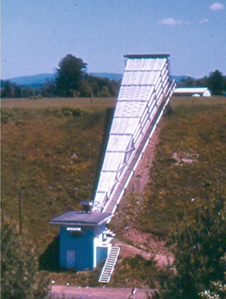
**Fig. 7.8** The “Little Big Horn” at the NRAO in Green Bank, WV. It measures the absolute flux density of the strong source Cassiopeia A at 21 cm wavelength once a day when the source drifts through the beam. Over many years, an accurate measure of the secular decrease in Cassiopeia’s intensity was also obtained (NRAO/AUI/NSF)
