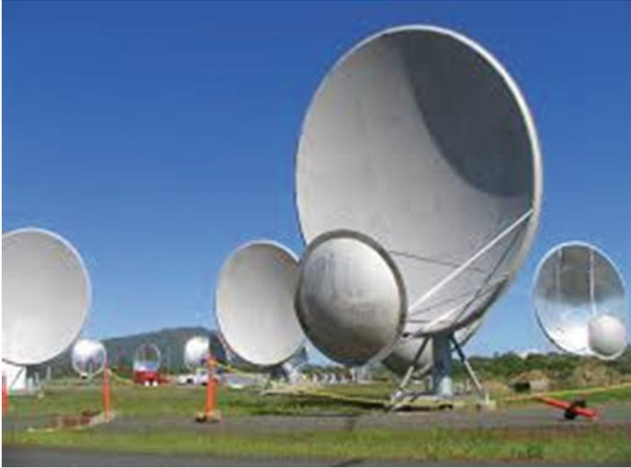
**Fig. 7.11** Dual-reflector offset antennas of the Allen Telescope Array (ATA). A shroud that shields the system from ground radiation supports the secondary reflector (Rick Forster, SETI Org.)
