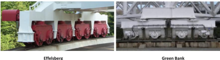
**Fig. 7.20** The lever systems for the bogies of Effelsberg and Green Bank telescopes
