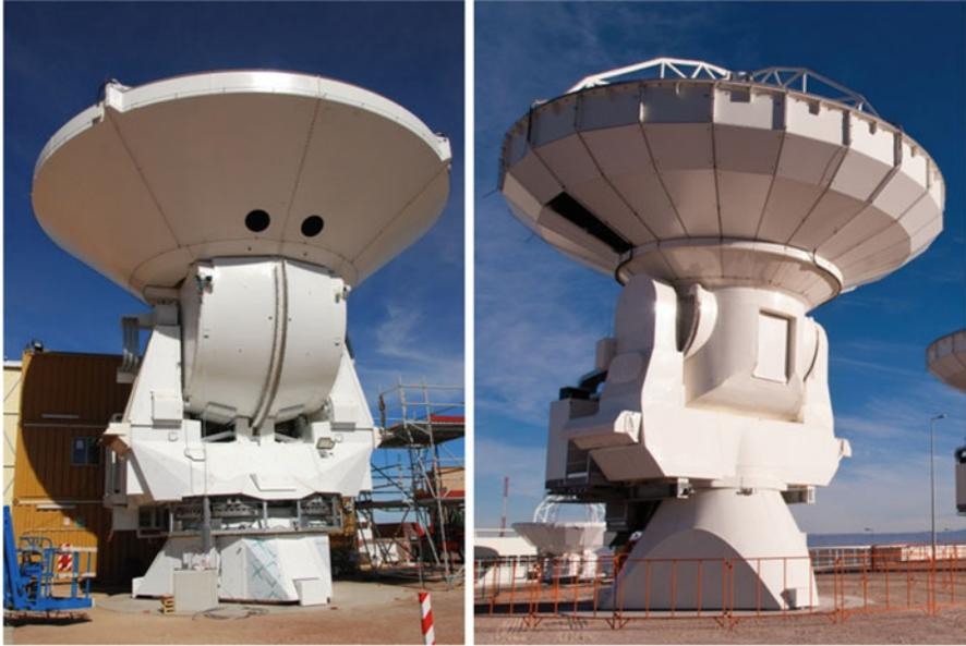
**Fig. 6.11** Antennas from AEM (*left*) and Vertex (*right*) at the ALMA Assembly site (ALMA-ESO/NAOJ/NRAO)
