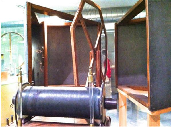
**Fig. 2.7** The original experiment, reconstructed after his move to the University of Bonn, is shown here while on display in the Deutsches Museum in Bonn (2013). The Ruhmkorff coil in front creates the sparks along the focal line of the cylindrical parabola on the left, which sends electromagnetic waves through the polarisation grid in the centre to an identical parabolic cylinder with receiver on the right (J. Baars, Deutsches Museum Bonn)
