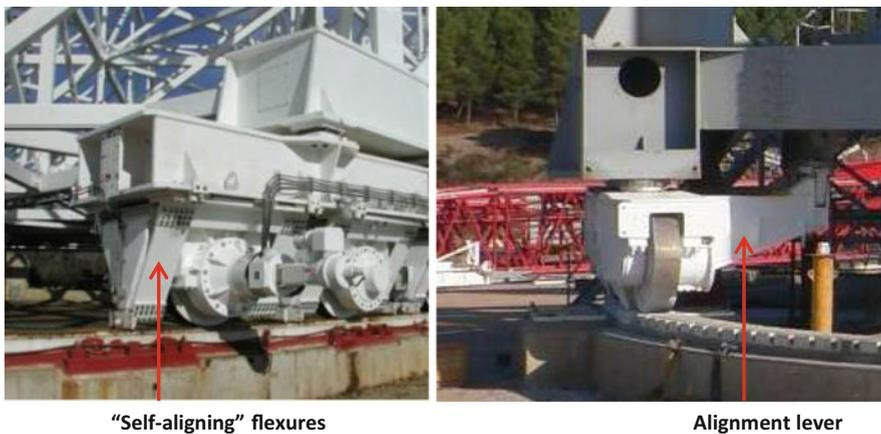
**Fig. 7.22** Two different design approaches for the wheel axes alignment. *Left*: GBT Green Bank Telescope; *right* SRT Sardinia Radio Telescope
