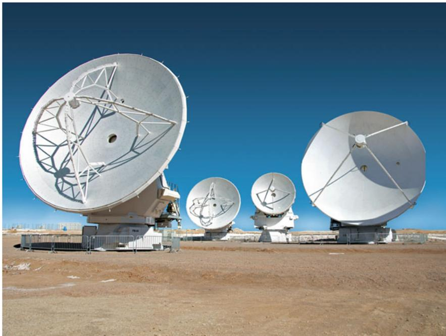
**Fig. 6.21** The four varieties of ALMA antennas. In foreground the 12-m antennas from Vertex (*left*) and Alenia-EIE-MT Mechatronics (AEM) (*right*). In background on right the 7-m antenna and on left the 12-m antenna from Mitsubishi [ALMA(ESO/NAOJ/NRAO), W. Garnier, ALMA]
