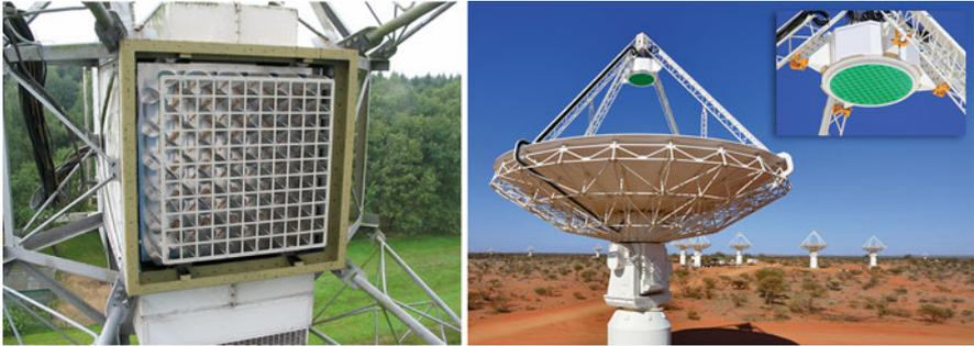
**Fig. 8.21** The Phased-Array Feed APERTIF in the focal plane of a WSRT antenna (*left*, ASTRON) and the Australian PAF (*green* feature in the inset) mounted on ASKAP in Western Australia (ASKAP/CSIRO)
