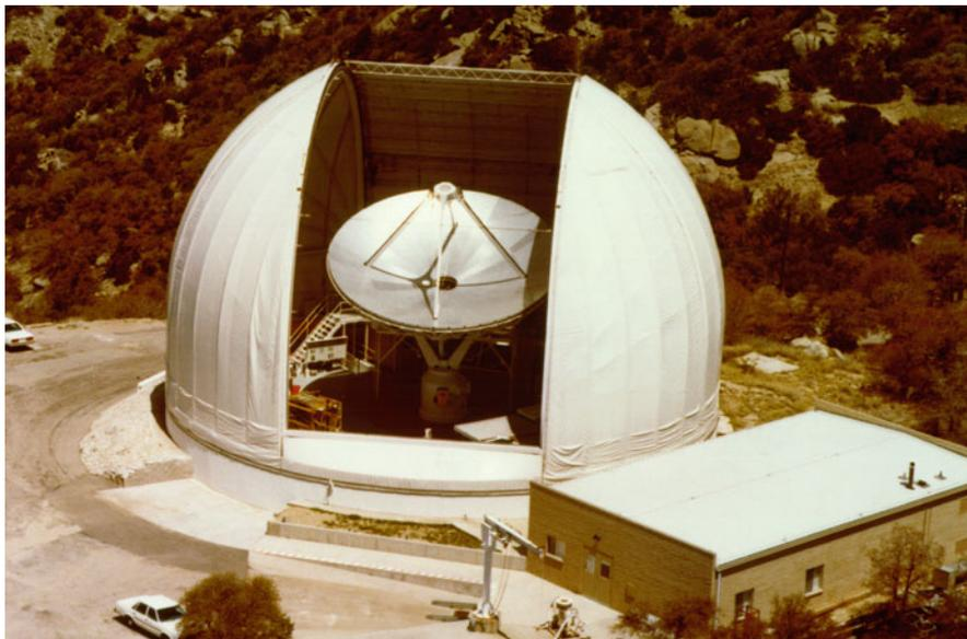
**Fig. 5.2** The second-generation surface of the NRAO mm telescope. The size of the dome allowed a diameter of 12 m. Surface panels from EESCO are supported by a truss-frame BUS designed at NRAO. The focal ratio was reduced to 0.42 and the system operates in Cassegrain mode (NRAO/AUI/NSF)
