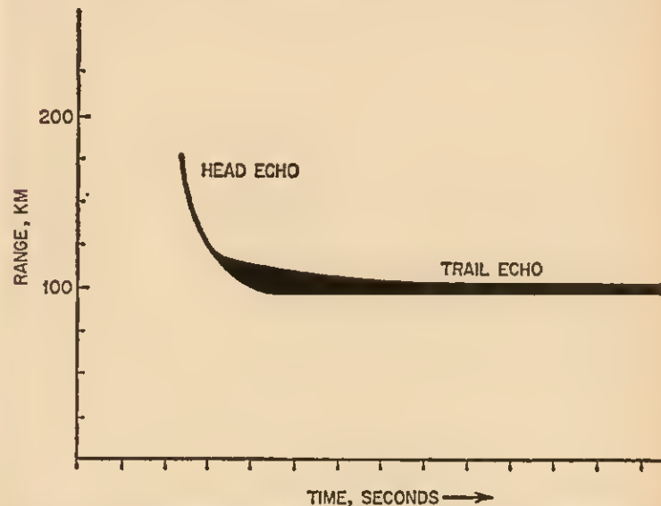
FIG. 6-1 Radar range-time record of a meteor for which echoes were obtained from the approaching head and afterward from the trail.
