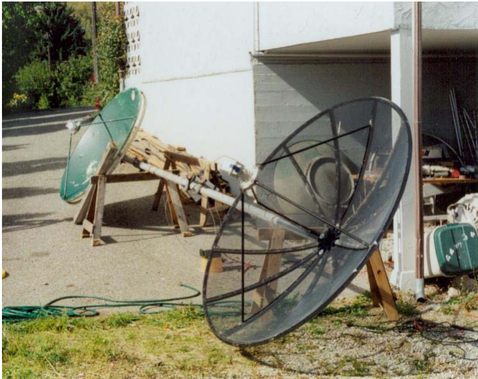
Figure 4: Trial version of the rigid interferometer. The antenna-mounting pipe is resting on the sawhorses used for the initial experiments.
