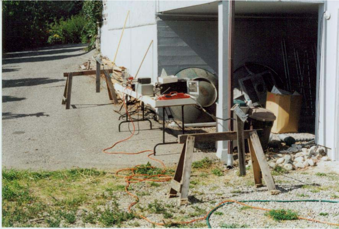
Figure 2: The Minimum Interferometer. The two LNA's are clamped to those vertical pieces of wood nailed to the sawhorses. The signals are carried to the table, where the rest of the electronics is located, by heliax cables. On the table are the additional amplifiers and the rest of the electronics and an old chart recorder. Parts of other experiments lie in the background. If this were a more permanent set up, the electronics would be indoors, and the waveguide openings would be covered with plastic sheet.
