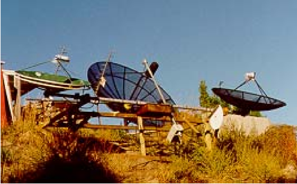
Figure 5: The rigid interferometer. The green, 5ft dish is on the left and the 6ft mesh dish is on the right. The receiver box is in the middle of the pipe. Also visible is the original 10ft dish and the yagis of the 408 MHz interferometer's west antenna.
