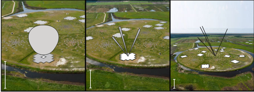
Fig. 14.1 Illustration of the individual tile beam (left), station SAPs (middle), and multiple CS beams (right). The bar in the bottom-left corner indicates how the picture is zooming out. Credit: Stappers et al., A&A , 530, 80, 2011, reproduced with permission © ESO
