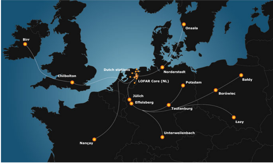
Fig. 11.2 LOFAR is composed of 24 core stations and 14 remote stations in the Netherlands, and 13 international stations (+1 planned)
