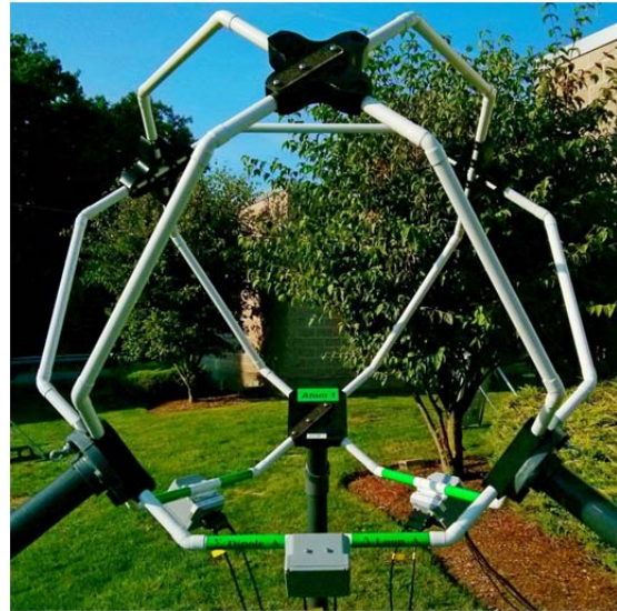
Figure 7. Atom 1 vector antenna at MIT Haystack Observatory. The three octagonal loops that form the vector sensor are painted copper tubing and the support posts are PVC. Each loop is 1m in diameter. This vector sensor is intended for ground testing only.
