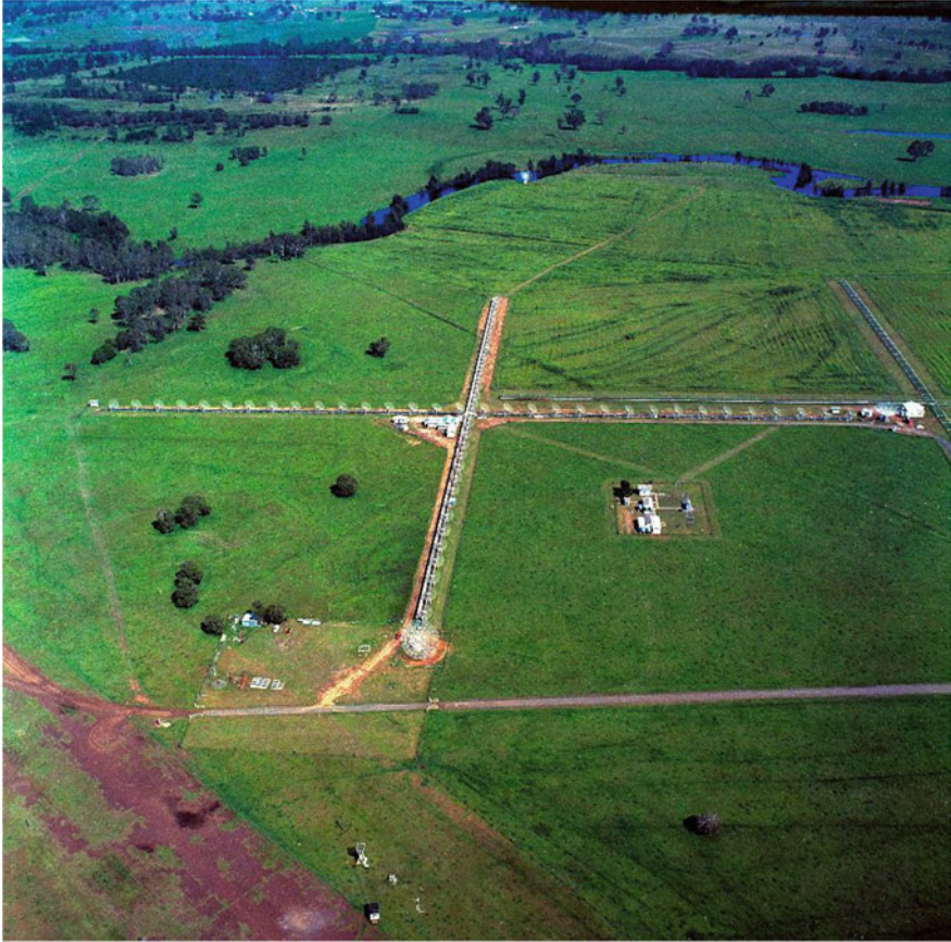
Fig. 4.22 An aerial view of the Fleurs Synthesis telescope in 1969. This used the original Chris Cross together with larger 13.7 m aerials to form a longer baseline and a much more sensitive synthesis instrument with a resolution of 45 and later 23 arcsec. The view is from the east looking west. The eastern 13.7 m aerial is visible on the immediate eastern end of the cross. The western 13.7 m aerial is visible just short of the creek line. The Mills Cross is visible to the right (CSIRO Radio Astronomy Historical Photographic Archives N9114-3)
