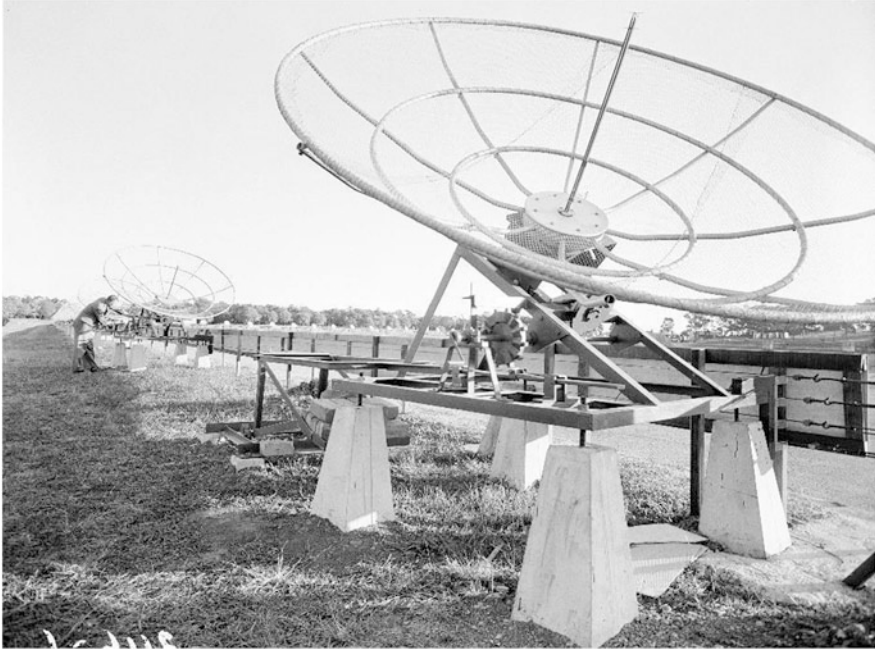
Fig. 4.9 The 16-element north-south arm of the solar grating array in July 1953 at Potts Hill. The array was located on the eastern bank of the No. 1 reservoir at Potts Hill. The view in the photograph is from the northern end of the array looking south. The E-W arm can be seen in the background on the southern bank of the reservoir. By combining data from the 32-element E-W arm of the array and the N-S arm, it was possible to construct a two-dimensional image of the solar radio emission at 1420 MHz (CSIRO Radio Astronomy Historical Photographic Archives 3116-1)
