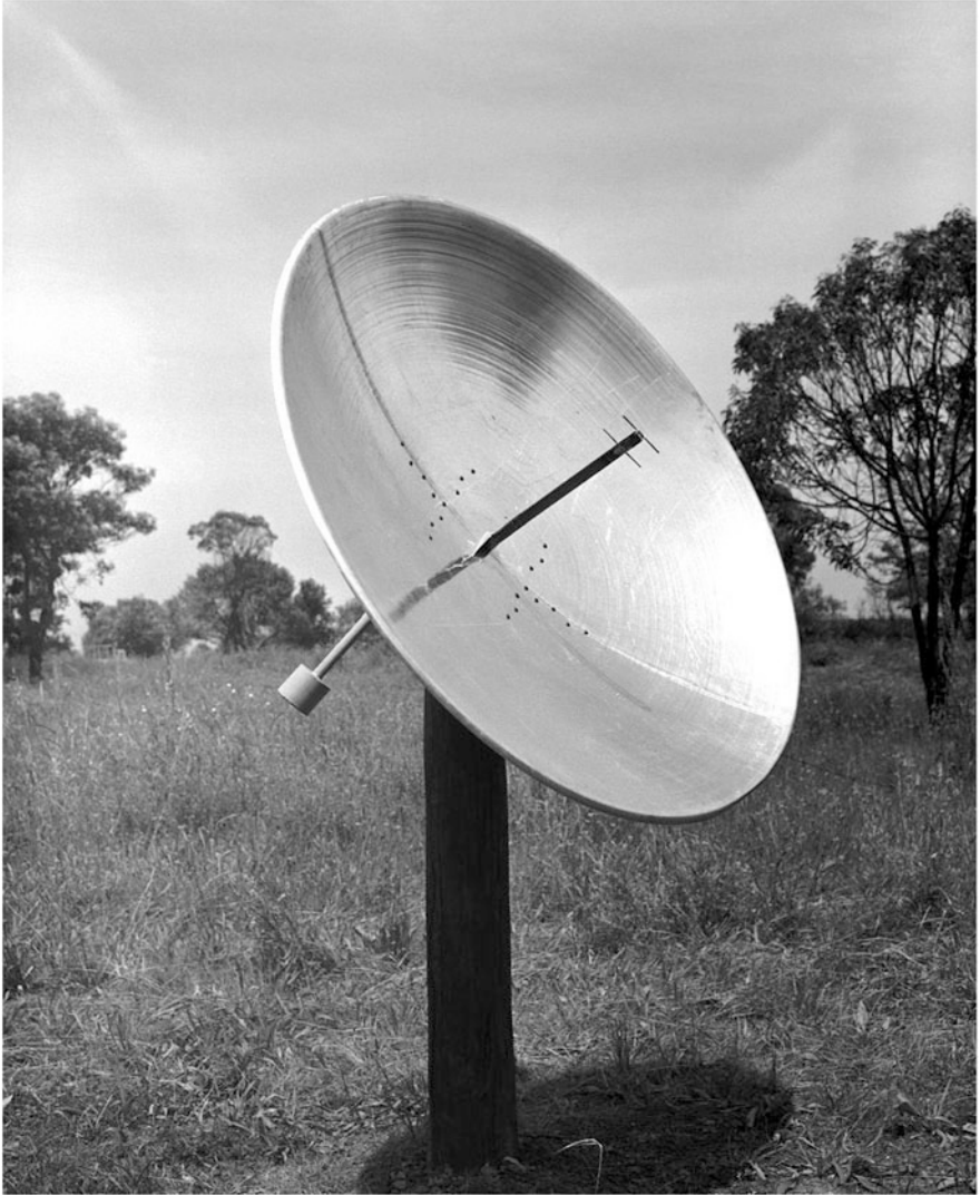
Fig. 4.6 A prototype dish for the solar grating array undergoing testing at Potts Hill in October 1950. (CSIRO Radio Astronomy Historical Photographic Archives 2294-1)
