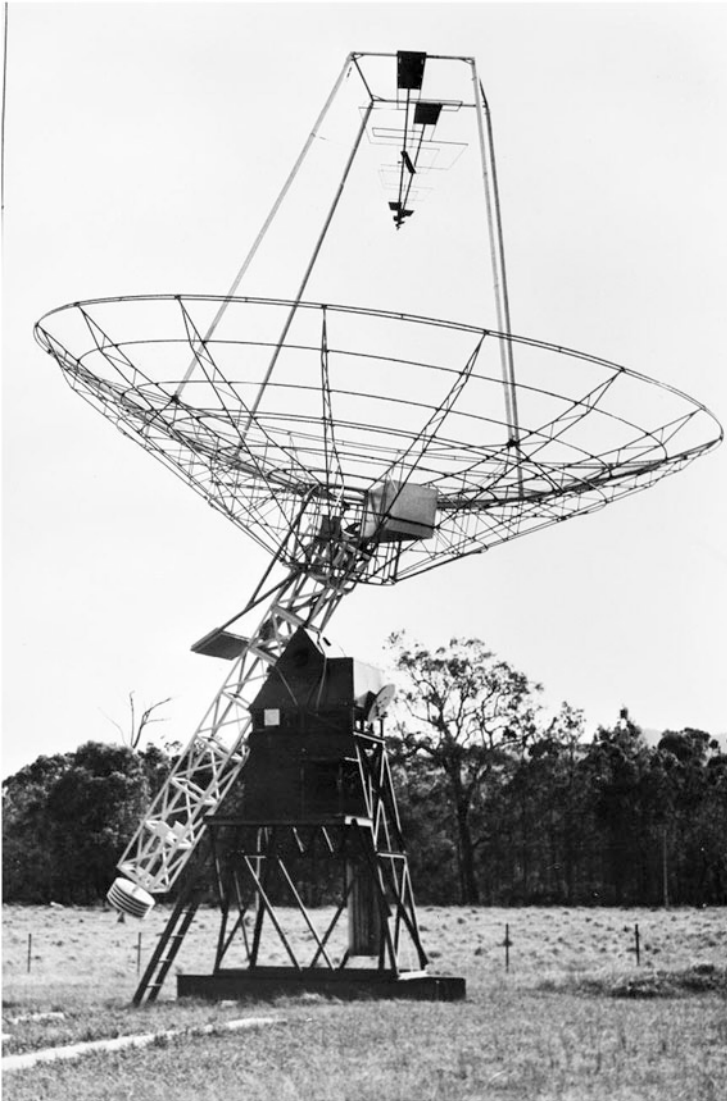
Fig. 5.16 The broadband 200–2000 MHz 30 f. parabolic aerial on an equatorial mount located alongside the three rhombic aerials at Dapto. This new instrument was used to extend the frequency coverage of solar burst analysis (CSIRO Radio Astronomy Historical Photographic Archives B7516-10)
