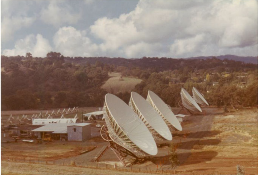
Fig. 6.11 The E-W-oriented five-element 18.3 m (60 ft) dish array at Heliopolis with the crossed-grating array in the background. This array operated at 10.7 GHz and produced a synthesis beam of 18.8 s of arc resolution. It was in use from 1972 to 1979 (Courtesy of the Goss Collection)
