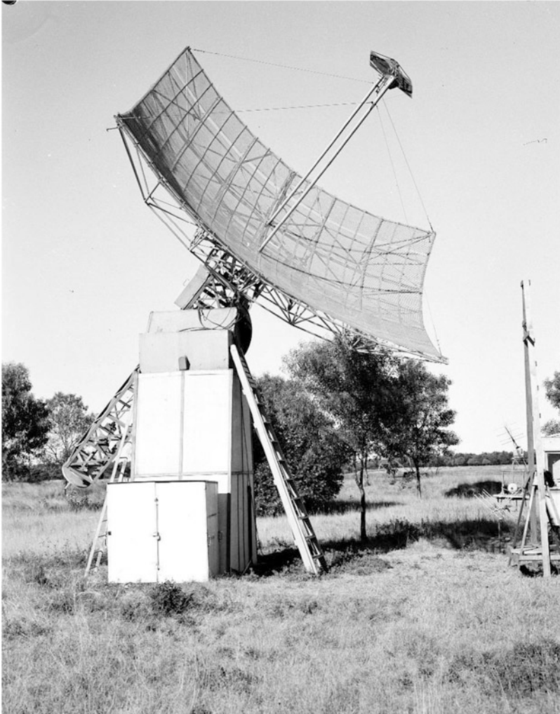
Fig. 4.3 The 16-ft \times 18-ft aerial at Potts Hill field station in May 1949. This aerial had been relocated from Georges Heights and was used by Christiansen to observe the partial solar eclipse of November 1948 and resulted in his first publication on radio astronomy (CSIRO Radio Astronomy Historical Photographic Archives B1903-1)
