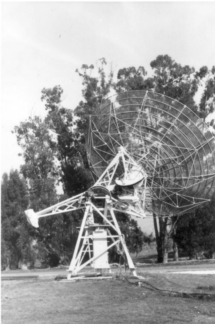
Fig. 6.10 One of the two 9.1 m (30 ft) equatorially mounted aerials used as an interferometer with the spectroheliograph array operating at 3.1 GHz. These aerials could be moved between several different foundations to vary the length and direction of the interferometer baselines (Courtesy of the Goss Collection)
