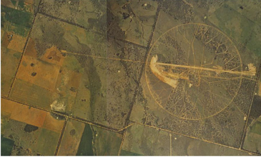
Fig. 7.5 An aerial view of Culgoora in the mid-1980s showing the newly bulldozed path of the east-west track of the Australia Telescope Compact Array in relationship to the original Radio-heliograph array. The westernmost station is the 6 km station of the Compact Array (CSIRO Radio Astronomy Historical Photographic Archives P14358-4)
