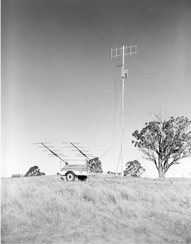
Fig. 3.5 The portable twin Yagi aerial system used by Mills in conjunction with a radio link to the 101 MHz broadside arrays to provide a variable interferometer spacing that allowed him to investigate the radio brightness distributions of the sources Centaurus A, Cygnus A, Taurus A and Virgo A. This photograph was taken in June 1952 and Mills presented his preliminary results during the 1952 URSI meeting (CSIRO Radio Astronomy Historical Photographic Archives B2786-6)
