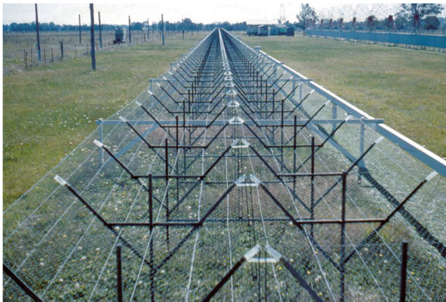
Fig. 3.14 A close-up view along an arm of the Mills Cross. To the right, a parallel arm of the Chris Cross is visible (CSIRO Radio Astronomy Historical Photographic Archives P12205-7)
