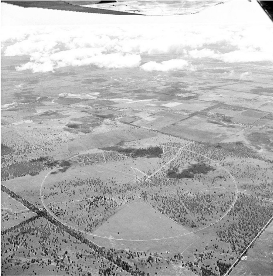
Fig. 5.31 An aerial view of Culgoora in 1964 showing the 3 km diameter ring of 96 aerials of the radioheliograph in 1964. The equipment buildings are in the centre of the circle . The trails for the transmission are visible as the cleared paths through the trees. The view is looking towards the northeast, with Yarric Lake Road showing on the bottom right (CSIRO Radio Astronomy Historical Photographic Archives B7660-25)
