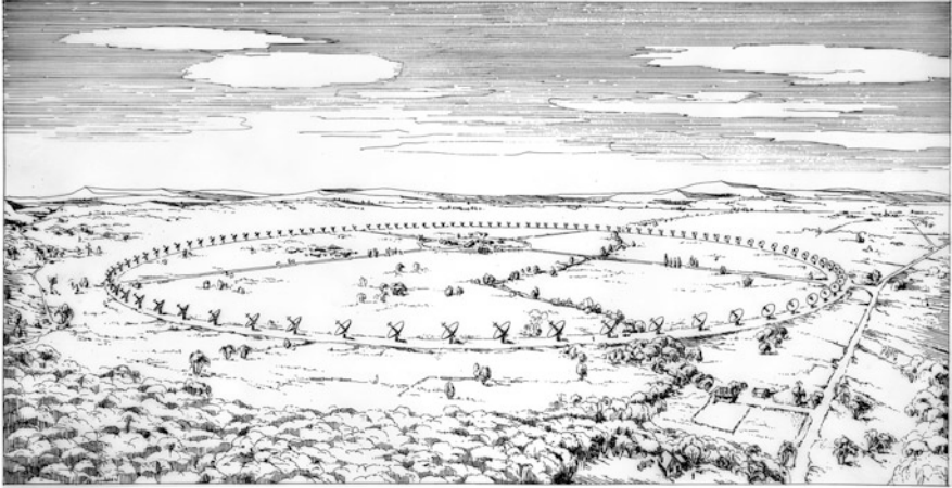
Fig. 5.19 An artist's impression of the Culgoora radioheliograph. It shows the intended 96 dishes, each a 13.7 m dish equatorially mounted in a circle 3 km in diameter (CSIRO Radio Astronomy Historical Photographic Archives B6636-22A)
