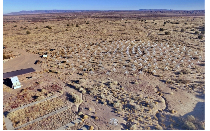
Figure 3. Aerial view of the LWA station at the Sevilleta National Wildlife Refuge. Most antenna elements are in a dense configuration towards the right of the image. A test antenna, is visible at the bottom. The signal processing hardware is contained within a modified, radio frequency shielded shipping container, visible in the left of the image.
