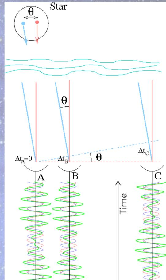
Figure 9: Telescopes A and B being close together receive beats almost at the same time resulting in a high degree of correlation. Telescopes A and C being further apart, do not receive beats at the same time and the correlation is low.
