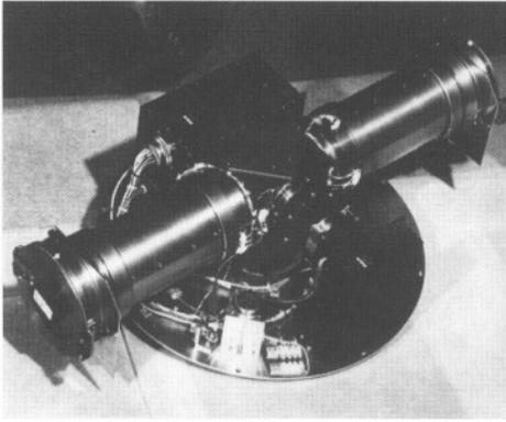
Figure 2.12a Cliff Anger's scanning instrument aboard the ISIS-2 Satellite: C. D. Anger.
