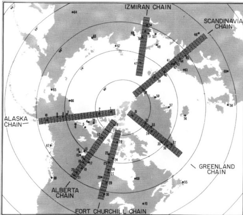
Figure 3.7 Six IMS meridional chains of magnetometers: B.-H. Ahn, Y. Kamide, and S.-I. Akasofu (1984).
