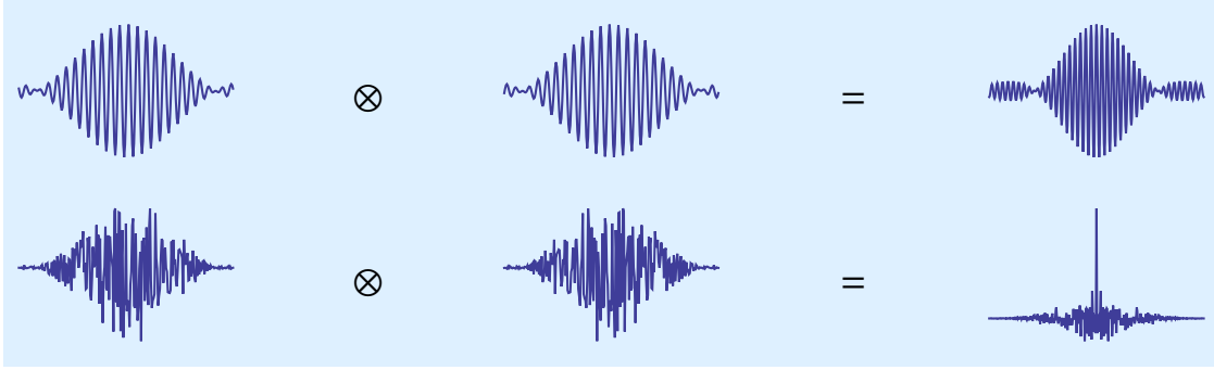
Figure 2.1: An illustration of an energy bundle and its detection using a matched filter. It consists of a waveform h(t) shown on the left, which can be simple or complicated. The remainder of the figure illustrates how this bundle of energy can be detected using a matched filter, which consists of a convolution (represented by \otimes ) with a time-reversed and conjugated version h^*(-t) (illustrated in the middle), with the result equal to the autocorrelation of h(t) (shown on the right). This autocorrelation can be sampled at zero lag, and the resulting value represents a filtered sample of the thermal noise. Various types of h(t) can be used as the basis for an energy bundle, but arguably the most useful are the segment of a sinusoid (on top) and the segment of a noise-like signal (shown on the bottom).
