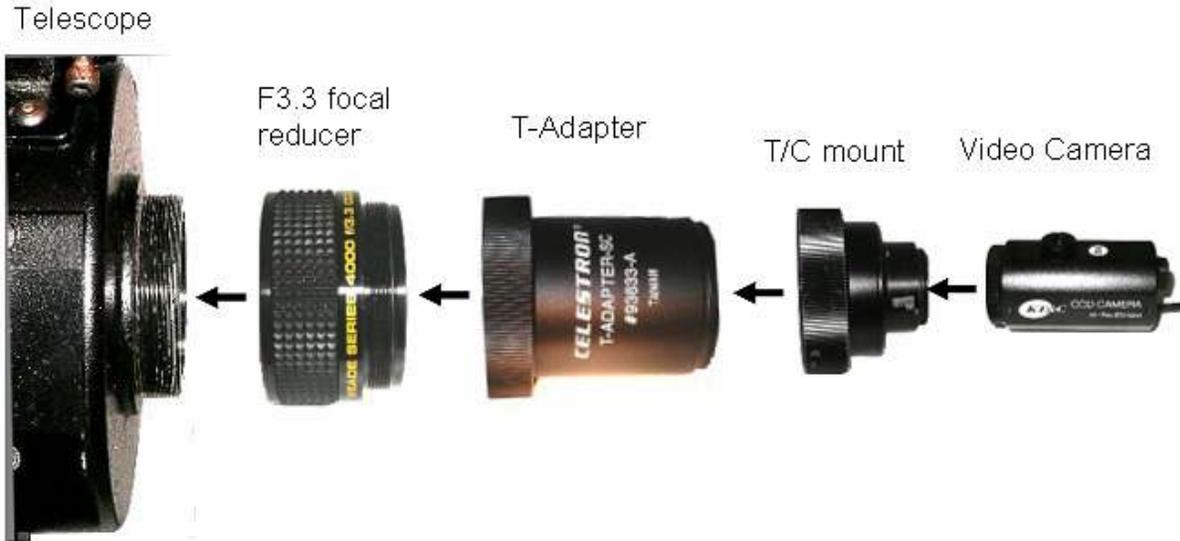
Figure G-4. Video camera adapted to telescope with f.3 focal reducer and T-adaptor.
