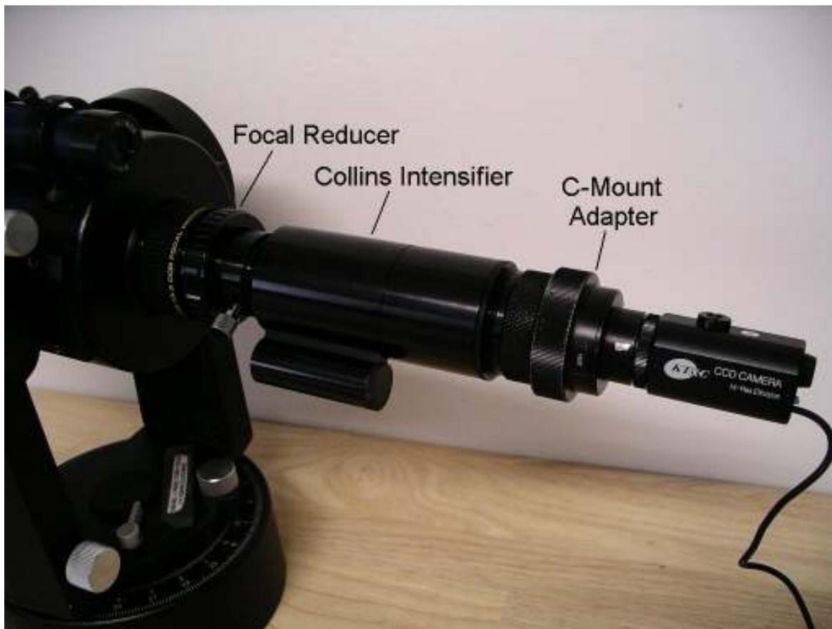
Figure 6.9. PC-164C camera attached to Collins I<sup>3</sup> Image intensifier. The Collins I<sup>3</sup> piece is attached to a f3.3 focal reducer at the back of the telescope. The Collins I<sup>3</sup> is powered by a 3V lithium battery with its holder attached to the bottom of the Collins tube.
