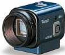
Watec 902H2 Ultimate: Several electronics and security company suppliers carry this camera, which retails for about \$325. The Watec 902H2 Ultimate has the same sensitivity as the Supercircuits PC164CEX-2, 0.00015 lux but has a larger 1/2" CCD chip, providing a larger field of view, plus has adjustment controls for shutter speed, manual gain control and Gamma correction.
