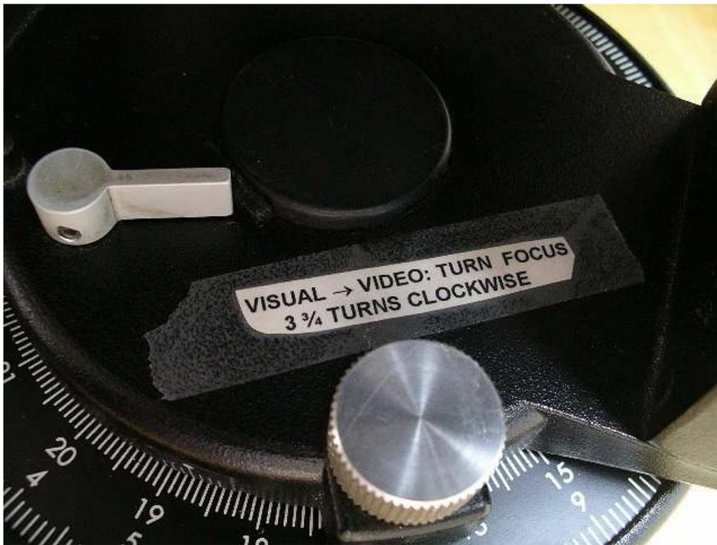
Figure 6.7b. Reminder note on telescope base to achieve rapid focus
