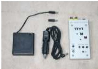
This unit manufactured in Japan by Tsutomu Hayamizu and is used with the GHS15-clock to produce an overlay of GPS time on video. For more about the units and sample screen shots and ordering information see: <http://www2.synapse.ne.jp/haya/ghstivi/ghstivi.html>
