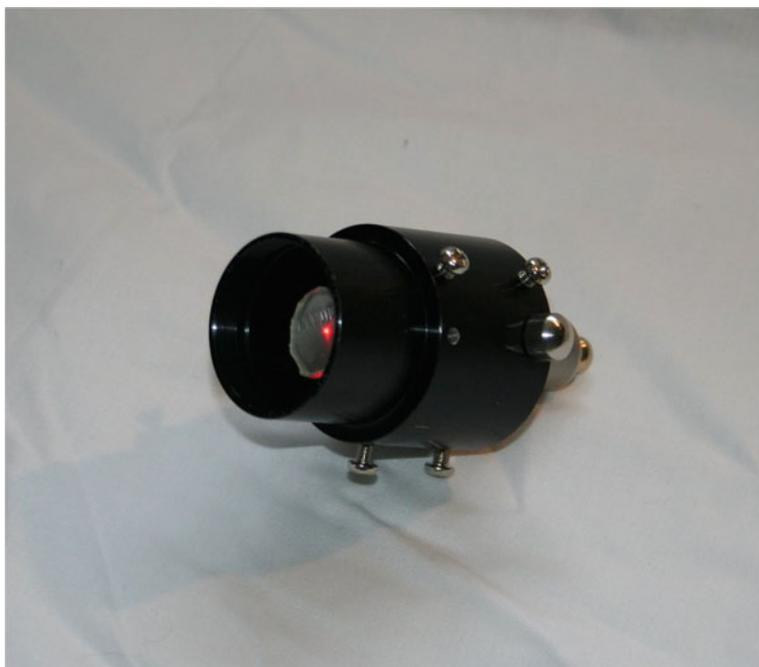
**Figure 12.18.** Homemade laser collimator.
