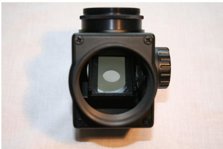
**Figure 16.4.** Beamsplitter in place.
