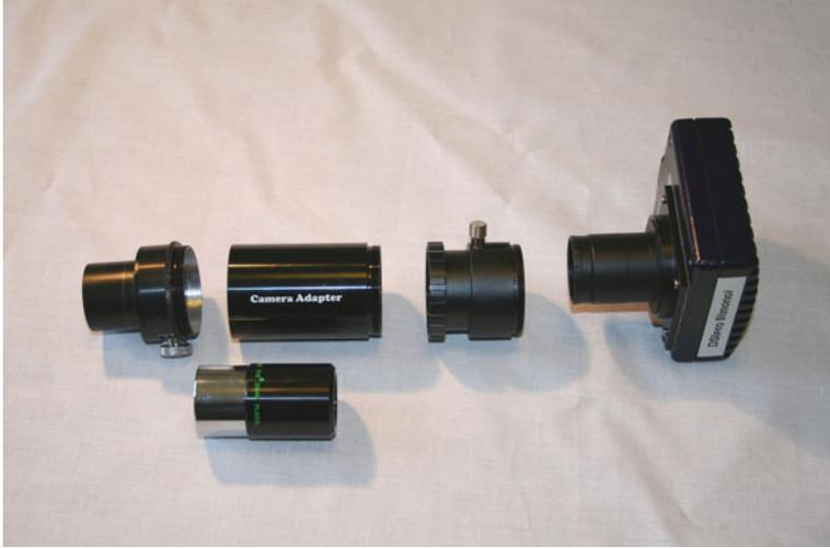
**Figure 14.12.** Components for adding a transmission grating slit.
