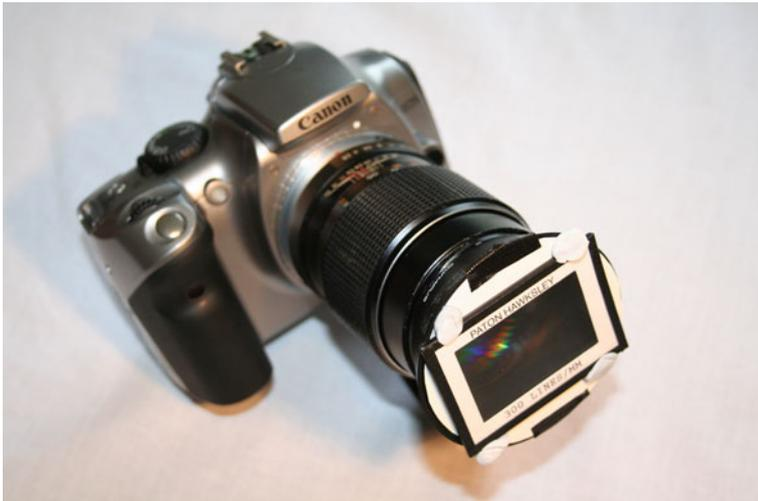
**Figure 6.6.** P-H grating mounted on a 135 mm telelens.
