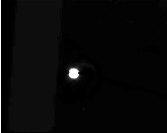
**Figure 16.11.** Image of star close to focus from the split mirror guider.
