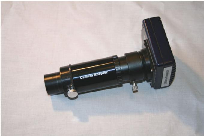
**Figure 14.13.** Grating with slit assembly.
