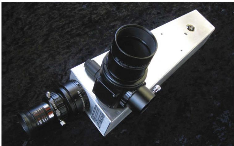
**Figure 8.8.** The Baches spectroscope. (Courtesy Baader.)
