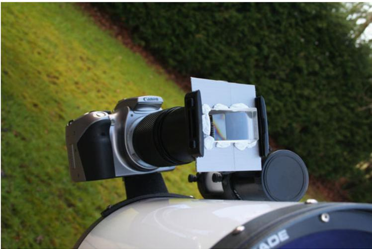
**Figure 6.1.** Mounting an objective prism.
