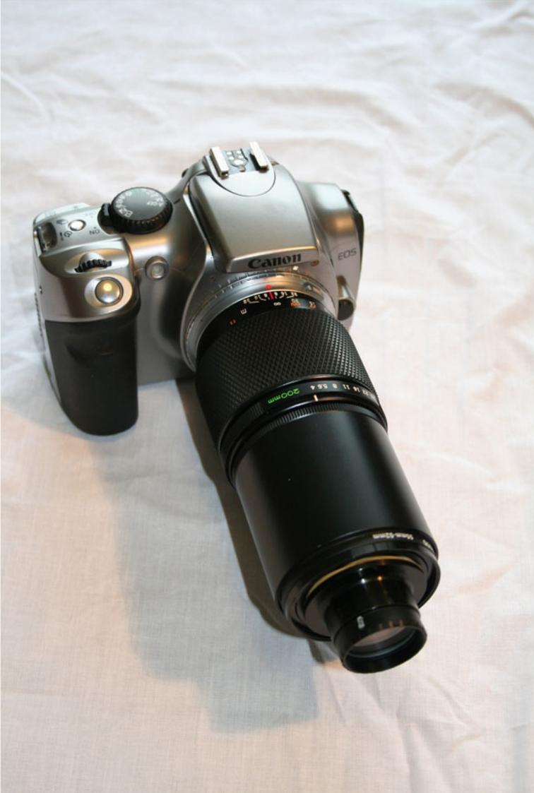
**Figure 14.1.** SA100 objective grating mounted on 200 mm telelens.
