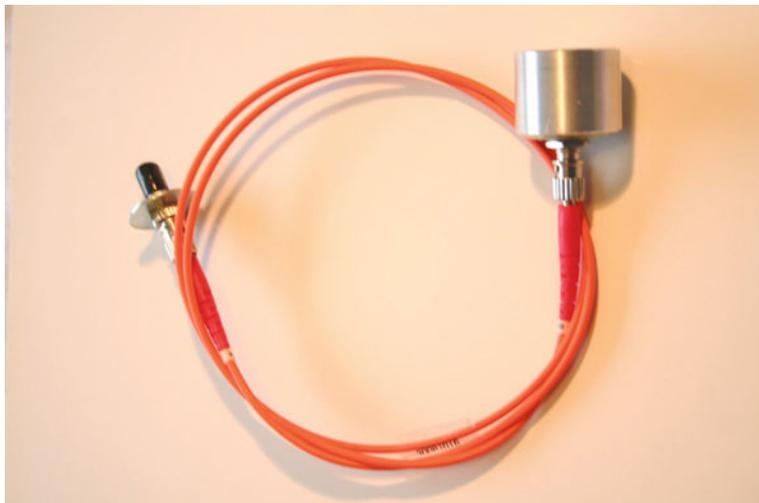
**Figure 15.17.** Standard fiber optic cable fitted to 1.25" nosepiece.
