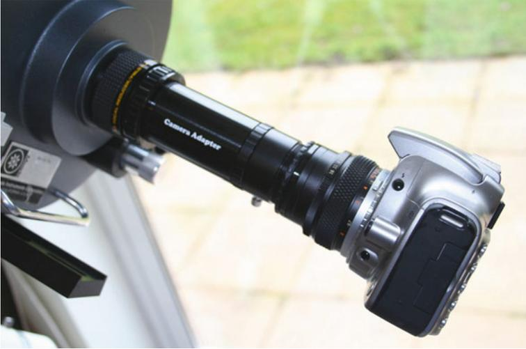
**Figure 7.6.** Final assembly of eyepiece projection with filter grating.
