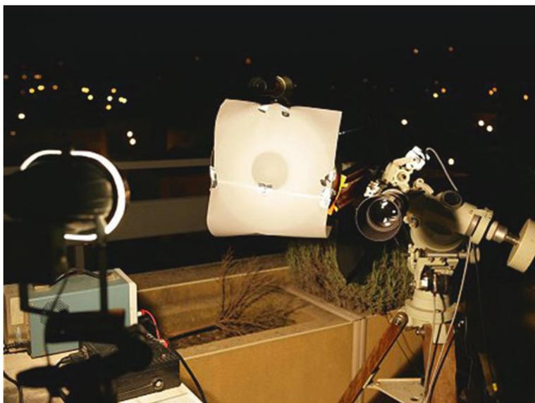
**Figure 9.7.** Taking a flat with a diffuser and halogen lamp. (C. Buil.)
