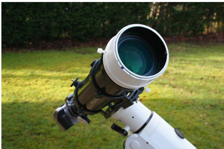
**Figure 13.3.** A 4° objective prism on an ED80.
