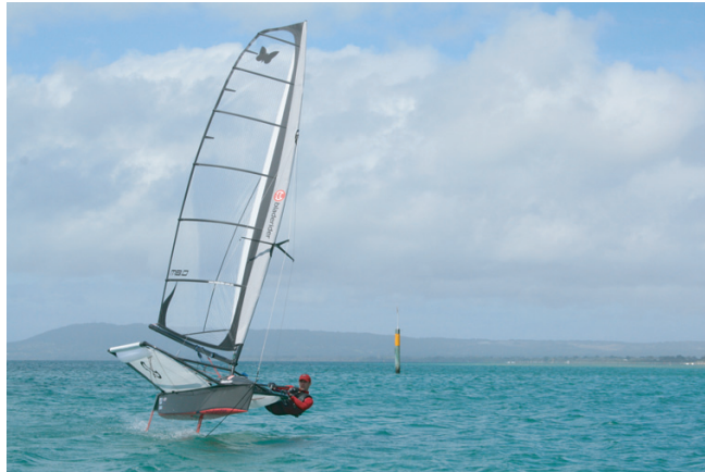
FIGURE 188 The moth sailing class: a 30 kg boat that sails above the water using hydrofoils , i.e., underwater wings (© Bladerider International)
