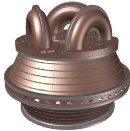
Fig. 7. The new HIT-SI3 experiment that is beginning operations. The three coplanar helicity injectors will provide flexibility in phasing that could enable plasma current profile control by varying the fluctuation profile required for IDCD, and also lead to bulk plasma rotation when the injectors are phased appropriately.
