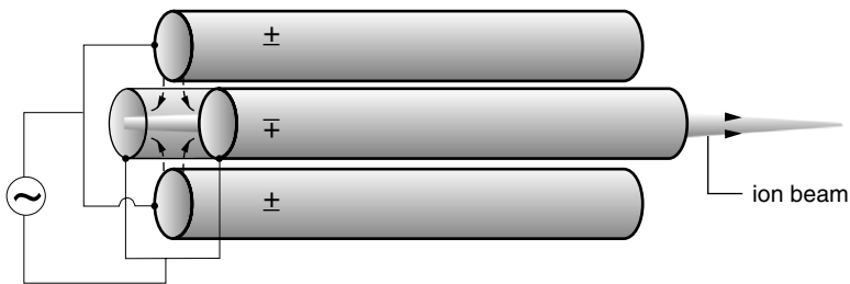
Figure 12.3 The Paul high-frequency ion mass filter
