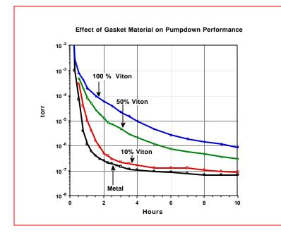
The pumpdown performance of the same unbaked system with varying linear percentages of metal and elastomer gasketing show that a small percentage of elastomer gasket will only affect the performance marginally.
