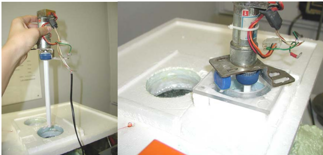
Fig. 21 Motor for crystal rotation
