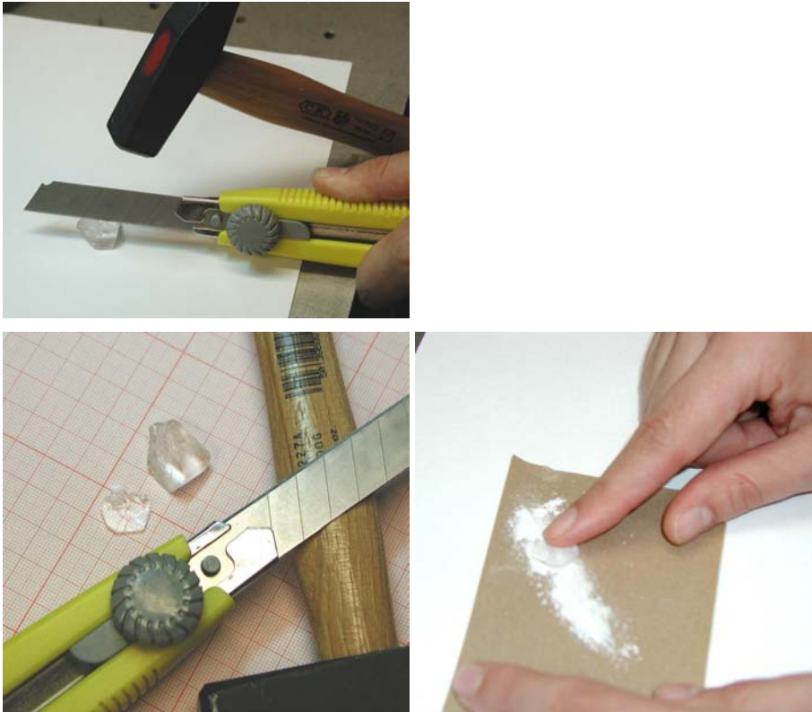
Fig. 16 crystal cleavage and thin slide polishing
