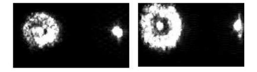
Figure 1: Nonlinear enhanced back-reflected scattering from the ferroelectric crystal surface as seen on the screen with the hole (left side of each picture). On the right side is the specular reflected beam with a 'droplet' for two frames (separated by 1 sec) from the video.
