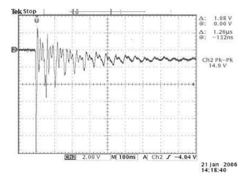
Figure 2: Electrical signal, picked up by the needle electrode from the laserilluminated spot of the LiNbO<sub>3</sub> crystal. Front edge of the electrical signal is in the nanosecond scale, damping oscillations are due to the reflections in the transmission line.
