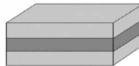
Figure 1. Structure of the PZT composites. The outer lightly coloured layers are the stainless steel, and the darker inner layer is the PZT.
